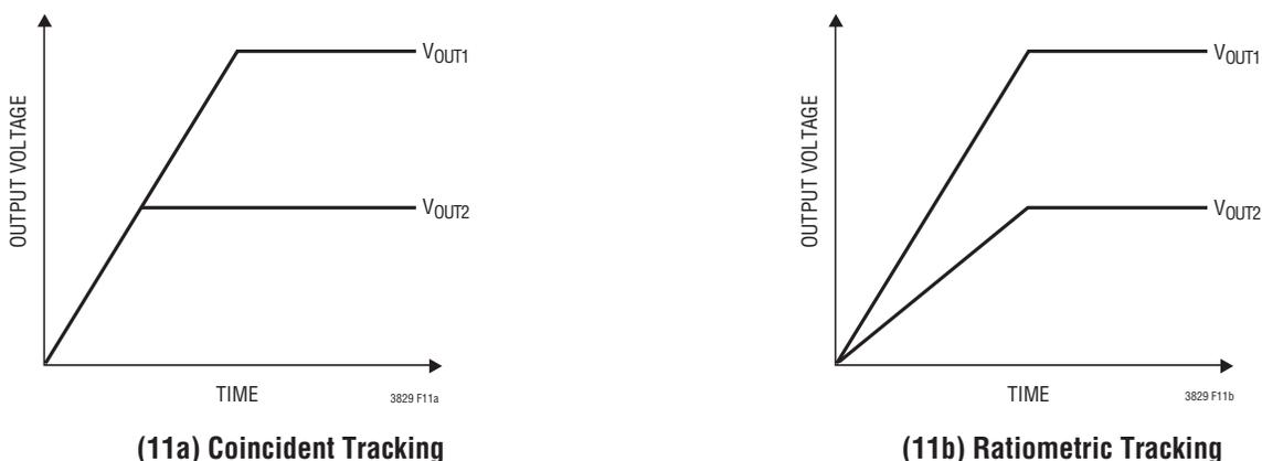
Figure 11. Two Different Modes of Output Voltage Tracking
