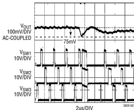
Load Step-Up (0A to 75A, 75A/ $\mu\text{s}$ )
