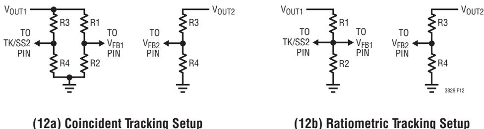
Figure 12. Setup and Coincident and Ratiometric Tracking
