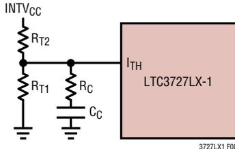
Figure 8. Active Voltage Positioning Applied to the LTC3727LX-1
