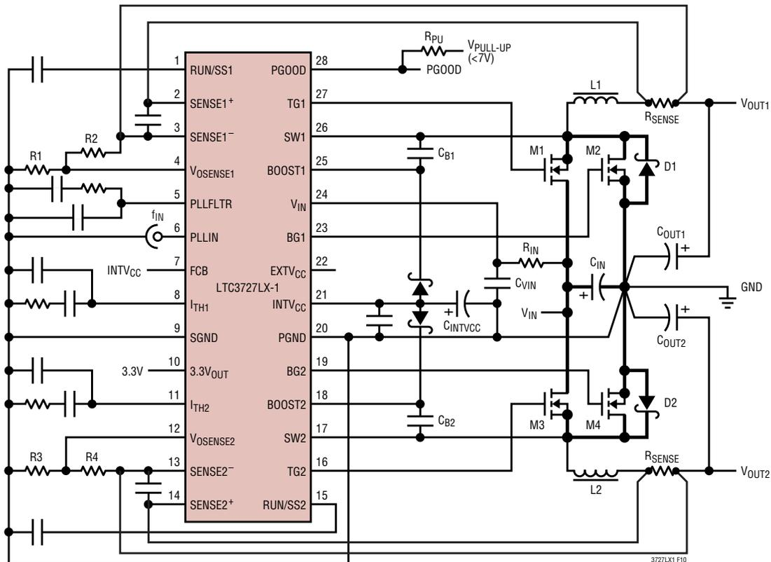
Figure 10. LTC3727LX-1 Recommended Printed Circuit Layout Diagram
