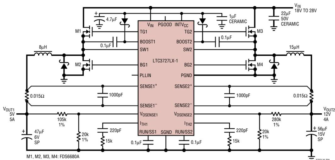
**Figure 1. High Efficiency Dual 12V/5V Step-Down Converter**
