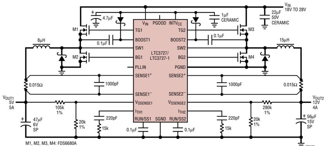
Figure 1. High Efficiency Dual 12V/5V Step-Down Converter
