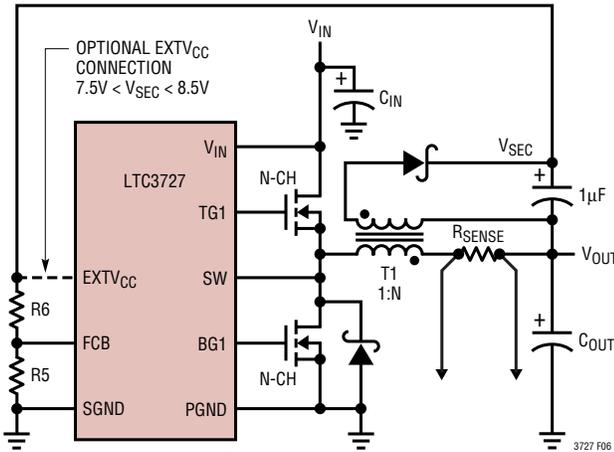
**Figure 6. Secondary Output Loop & EXTV<sub>CC</sub> Connection**
