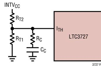
**Figure 8. Active Voltage Positioning Applied to the LTC3727**
