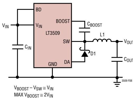
Figure 8. Supplied from V<sub>IN</sub>
