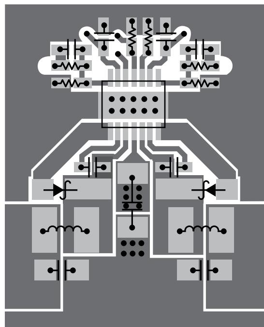
Figure 13. Sample PCB Layout (Top Layer Only)
