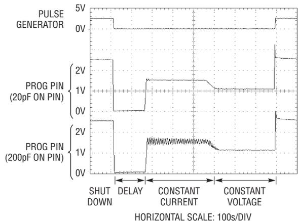
Figure 5. Stability Waveforms
