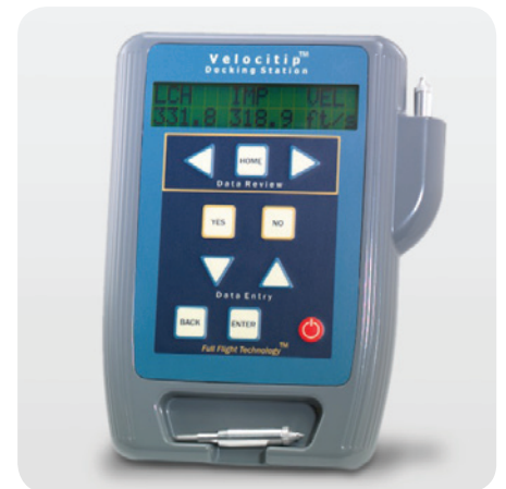
The VELOCITIP arrow tip is removed from the arrow and plugged into this docking station for data download.
