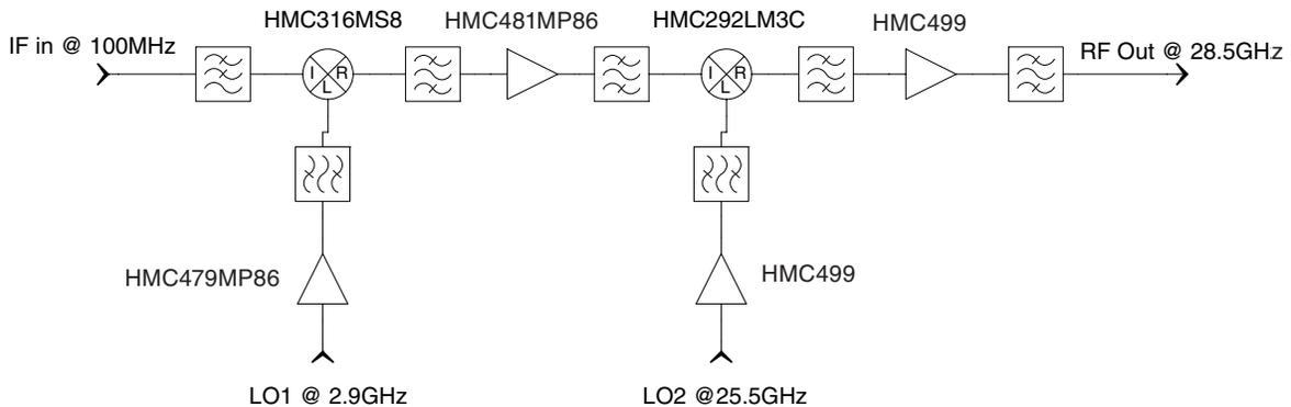
**Figure 8b** - Transmit chain using HMC292LM3C double-balanced mixer
