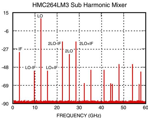
**Figure 7 (a)** - HMC264LM3 spurious response
