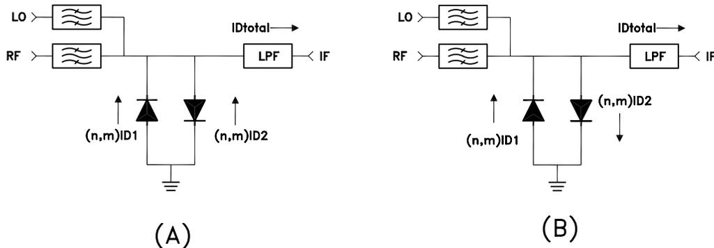
**Figure 2 -** IF current distribution for (a) odd order products, and (b) even order products.
