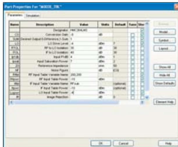
**Figure 6** - =SPECTRASYS= mixer parameters
