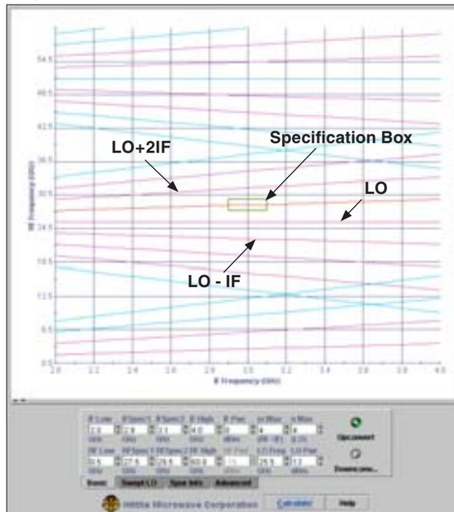
**Figure 4 - Sample of Hittite's Web-Based Spurchart Calculator Output**
