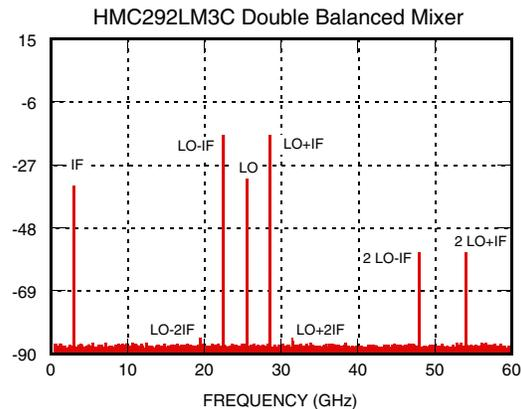
**Figure 7 (b)** - HMC292LM3C spurious response
