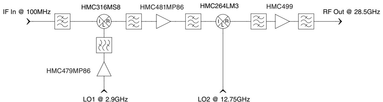
**Figure 8a** - Transmit chain using HMC264LM3 subharmonic mixer
