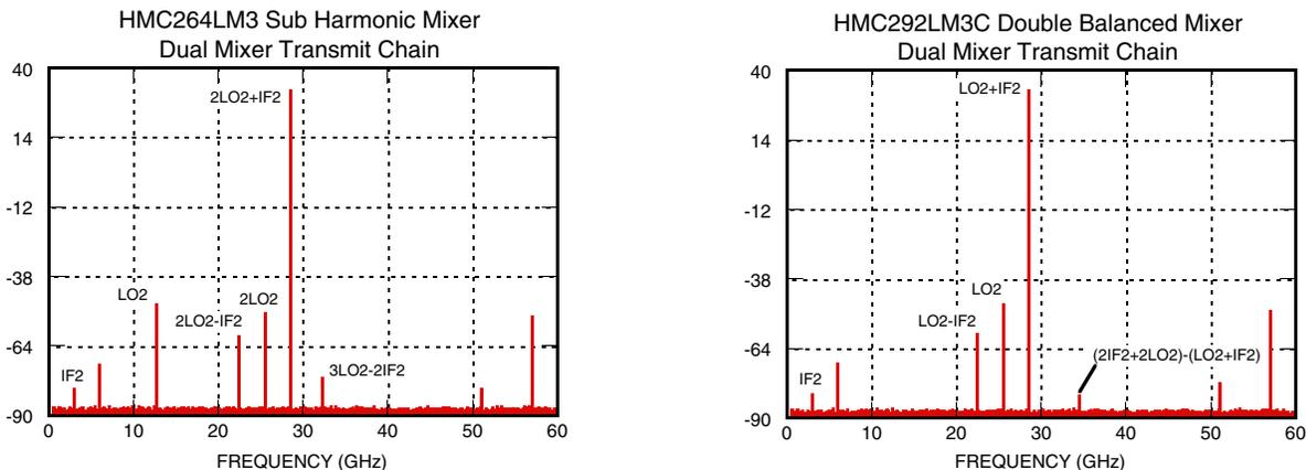
**Figure 9 (a)** - Transmit chain with subharmonic mixer
