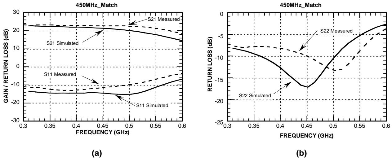
Figure 14 (a) 450MHz match S21 and S11, measured versus simulated.
