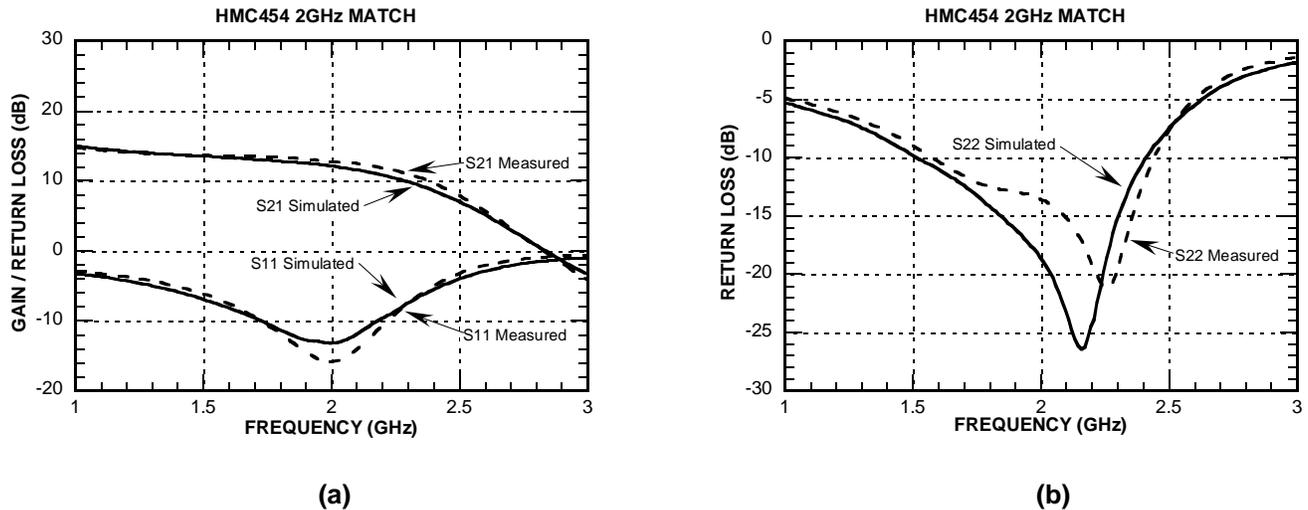
Figure 15 (a) 2140MHz match S21 and S11, measured versus simulated.
