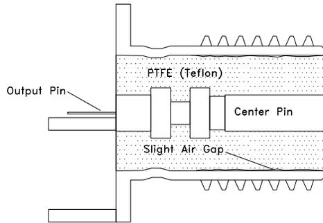
**Figure – 2 Cross Section of Edge Mounted Connector**
