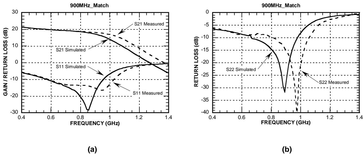
Figure 13 (a) 880MHz match S21 and S11, measured versus simulated.
