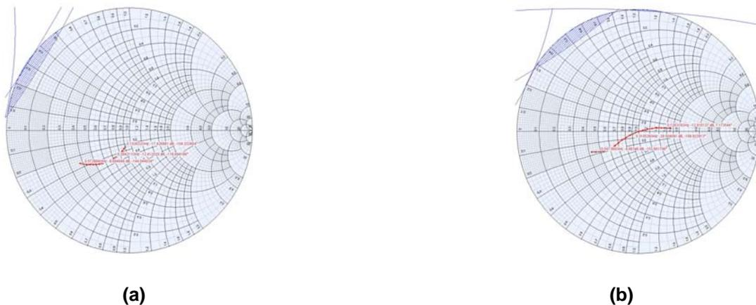
**Figure 12 (a) Input stability circles versus input matching network.
