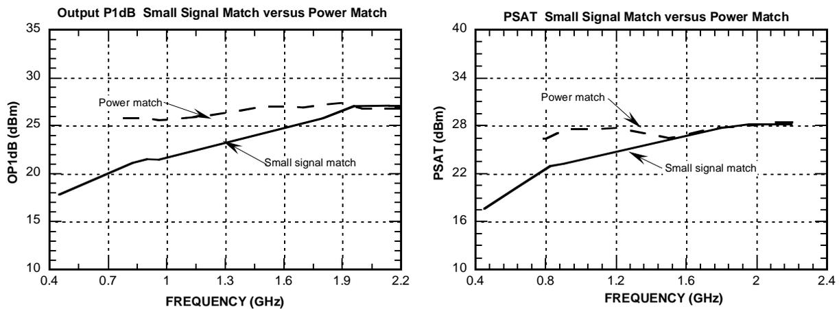
**Figure-16 (a) Large signal OP1dB versus small signal match
