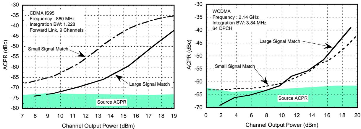
**Figure-18 (a) Large signal ACPR versus small signal match at 880MHz
