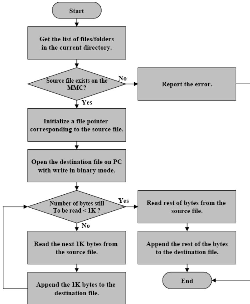
*Figure 10. Reading a source file from the MMC and copying it to the destination file*
