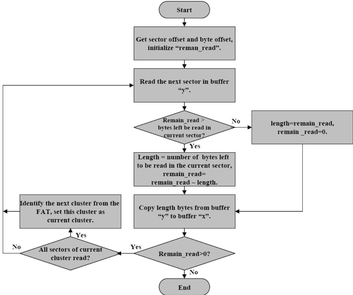
Figure 11. Reading a file from an MMC
