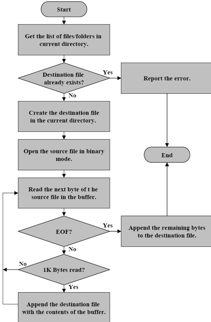
Figure 8. Copying a file “source” from a PC to a file “destination” on the MMC
