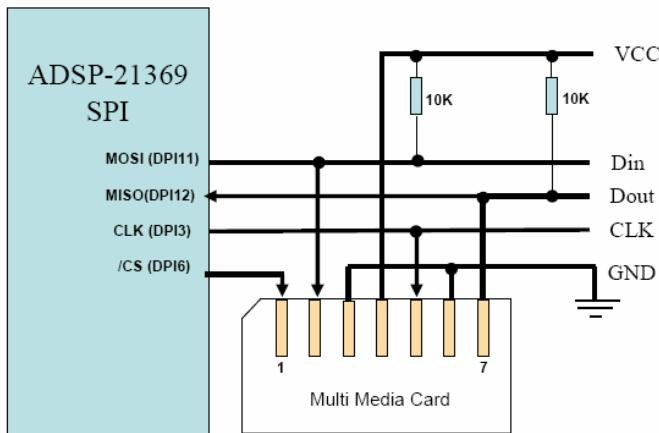
Figure 3. SHARC processor to MMC interface
