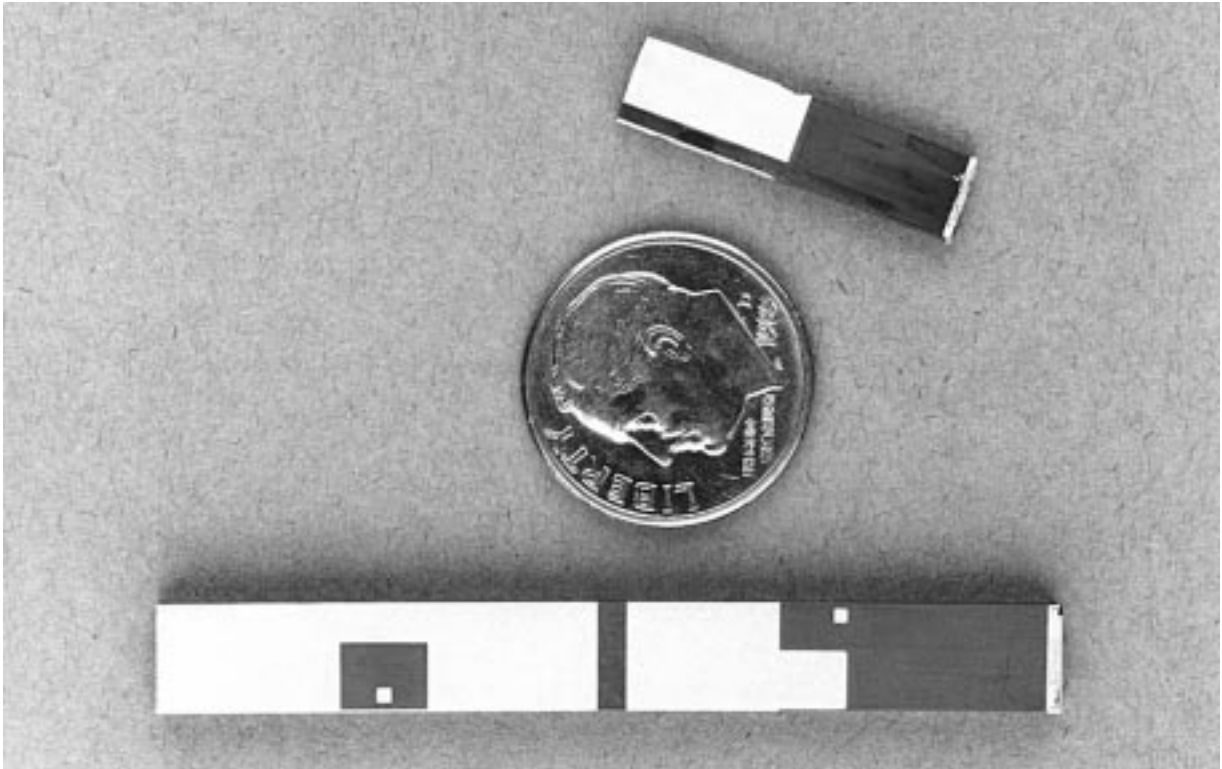
Figure 1. Piezoceramic Transformers Compared to a Dime for Size. 1.5 Watt (Photo Upper) and 10 Watt (Photo Lower) Units Are Shown. Devices Are Narrower Than Magnetic Transformers
