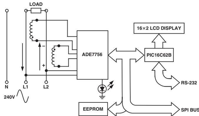
Figure 1. Simple Single Phase Watt-Hour Meter Block Diagram
