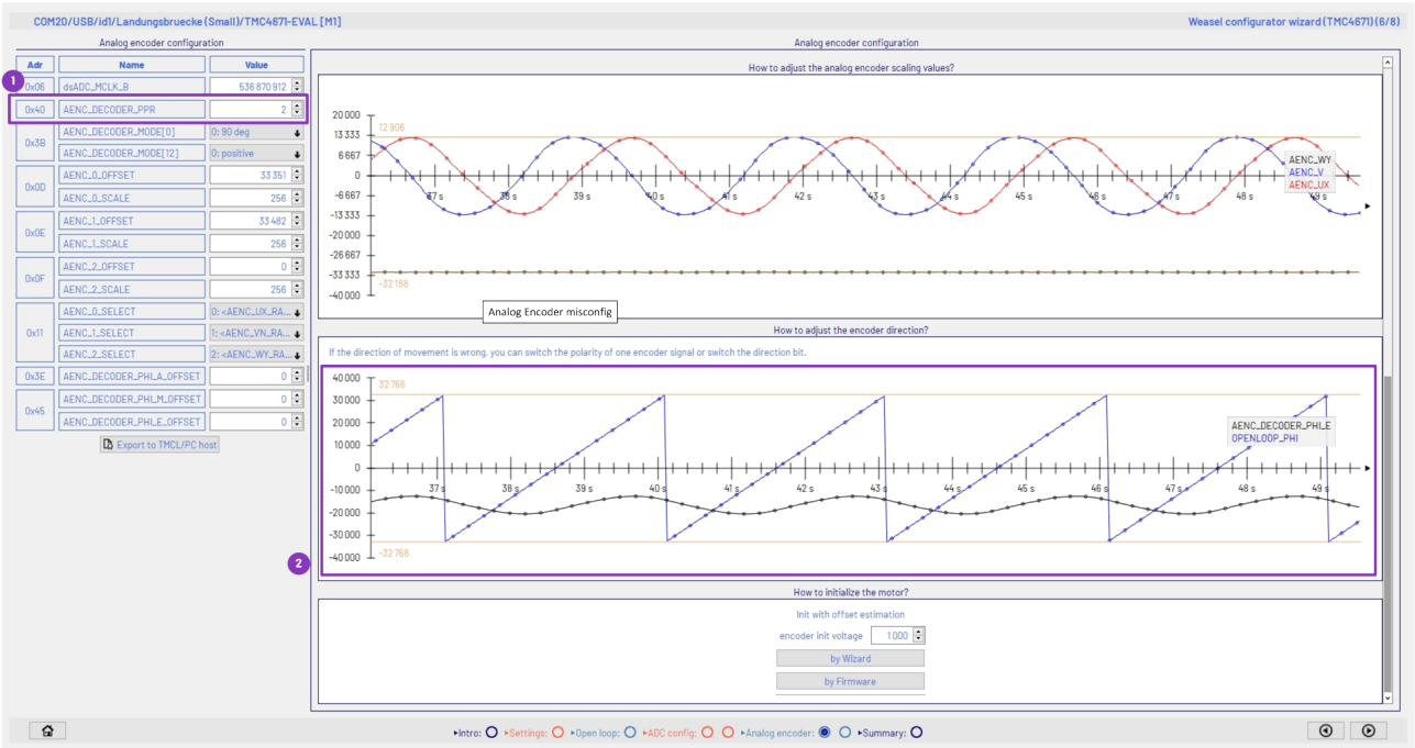
Figure 19: Analog Encoder Example of an Unusable Signal
