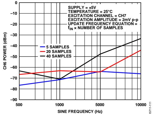
Figure 11. Analog Crosstalk in Adjacent Channels
