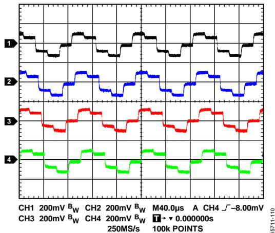
Figure 10. 10 kHz Sine Wave, 4 Channels at 200,000 UPS Using the AD5766/AD5767
