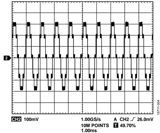
Figure 7. 1 kHz Sine Wave at 10,000 UPS Using the AD5766/AD5767
