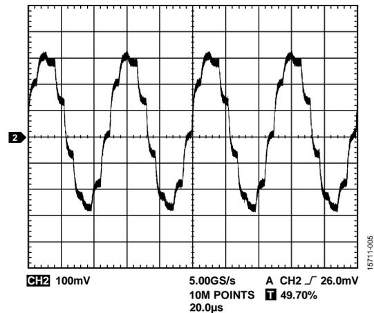
Figure 8. 20 kHz Sine Wave at 180,000 UPS Using the AD5766/AD5767
