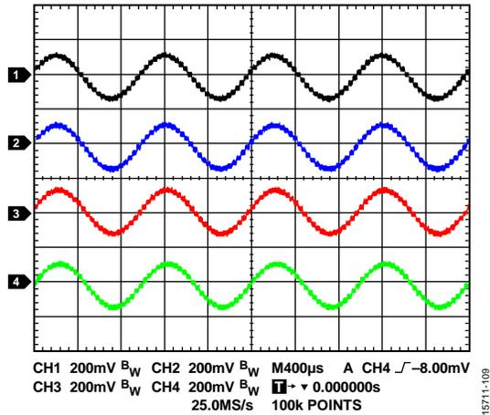
Figure 9. 1 kHz Sine Wave, 4 Channels at 100,000 UPS Using the AD5766/AD5767
