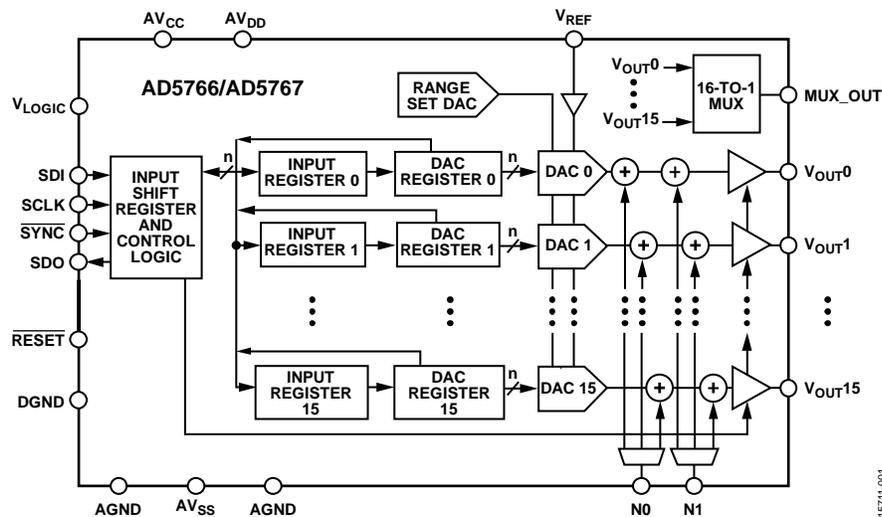
Figure 1. **AD5766/AD5767** Block Diagram
