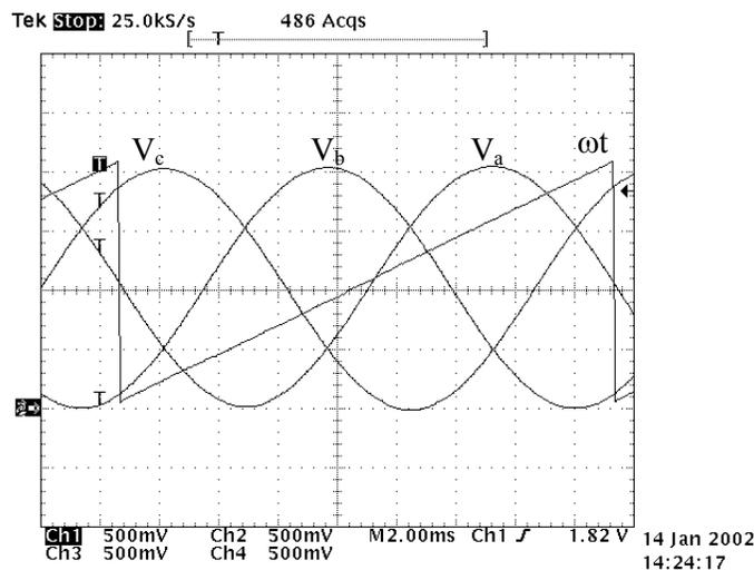
**Figure 3 Vector variable Vabc (the saw-tooth is the angle representation ranging from  $-\pi$  to  $+\pi$ )**
