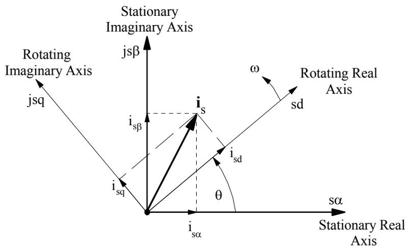
**Figure 2:** Relationship of current space vector components in stationary and rotating reference frames.
