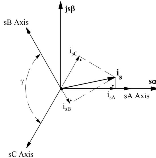
**Figure 1:** Relationship of stator current space vector and stator phase currents.
