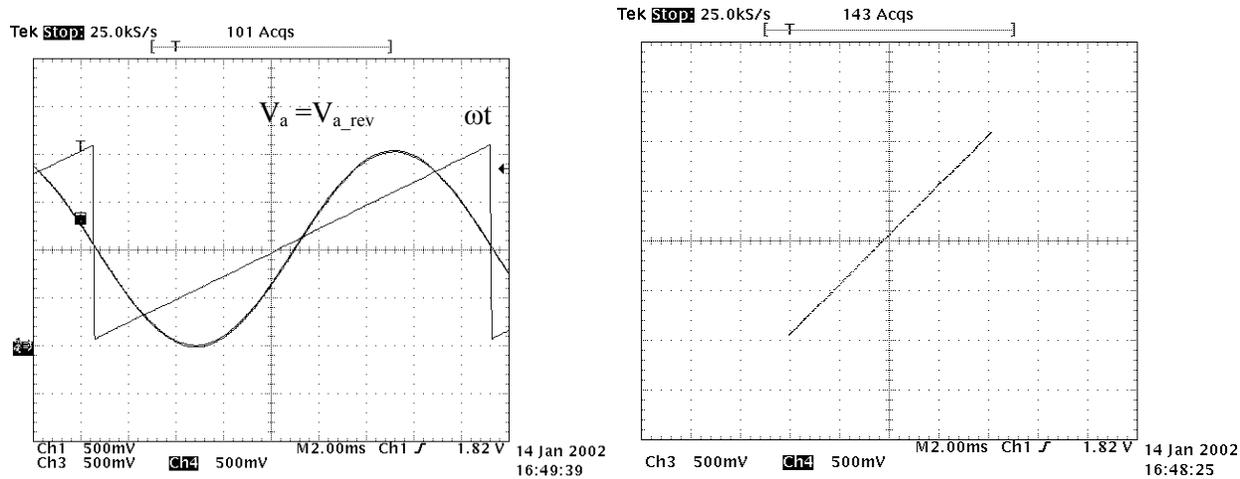
Figure 6  $V_a$  and  $V_{a\_rev}$  versus theta (left) and in xy representation (right)
