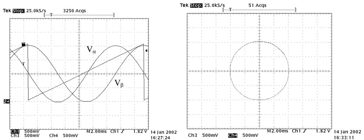
Figure 4 Vector variable Valphabeta versus theta (left) and in the \$\alpha\beta\$-plane (right)
