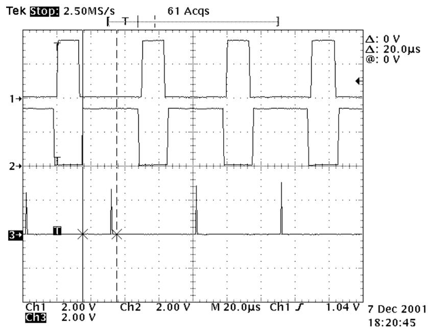
Figure 3 PWM outputs, Ch1: AH, Ch2: AL, Ch3: PWMSYNC
