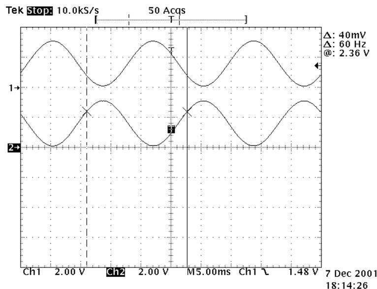
Figure 1 Filtered sine PWM outputs Ch1: AH, Ch2:AL
