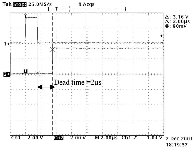
Figure 4 PWM outputs, Ch1: AH, Ch2:AL
