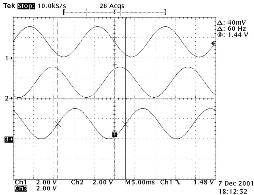
Figure 2 Filtered PWM outputs, Ch1: AH, Ch2: BH, Ch3: CH
