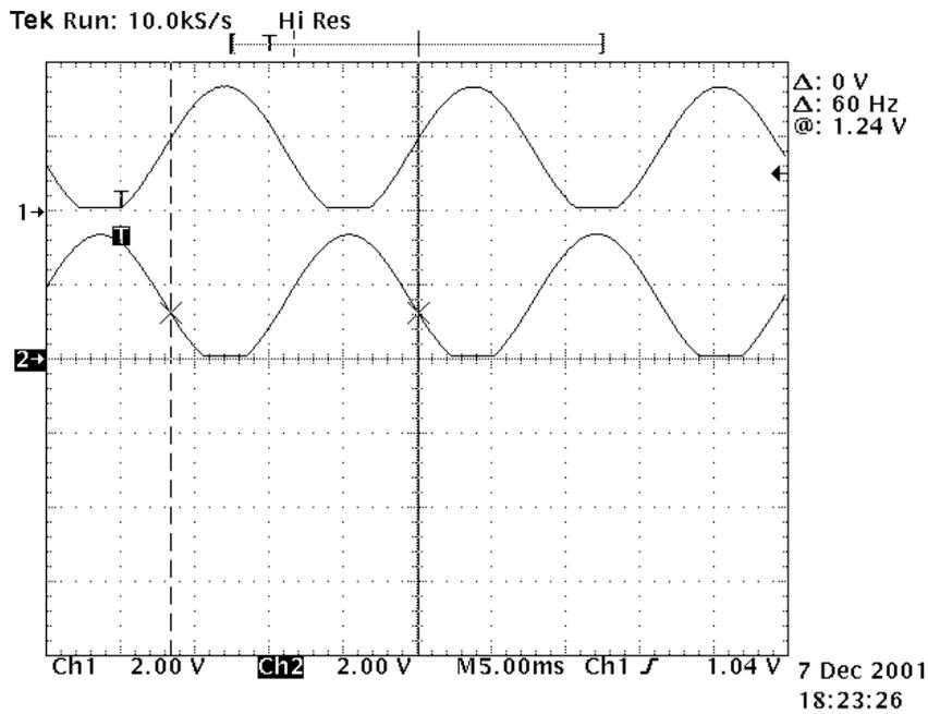
Figure 5 Filtered PWM outputs (over modulation) Ch1: AH, Ch2: AL
