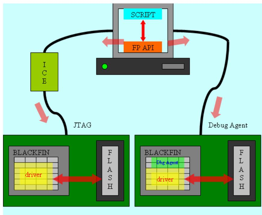
Figure 1: Communication Path Between Host PC Script and Flash Chip Via Flash Programmer API
