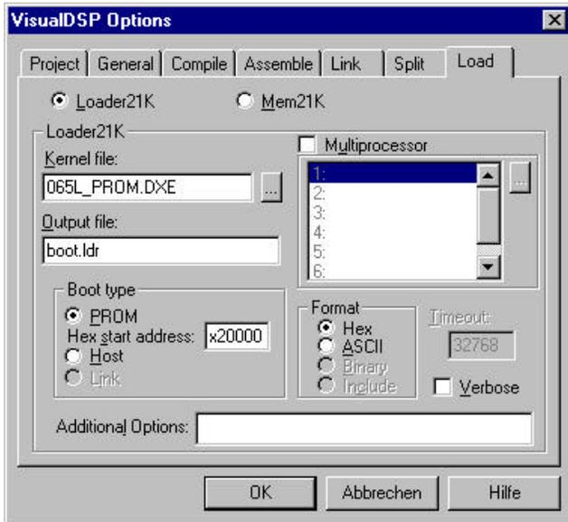
To provide a workaround the boot kernel of VisualDSP 4.1 sets the address line A17 in EIEP0 for all byte DMA reads<sup>1)</sup>. EPROMs greater than 1 MBit may be used, but then the entire boot image must start from 0x02.0000 on. Therefore an offset of 0x02.0000 has to be added when compiling the project. Just specify a “Hex Start Address” of 0x02.0000 in the VisualDSP “Load” Property Page.
