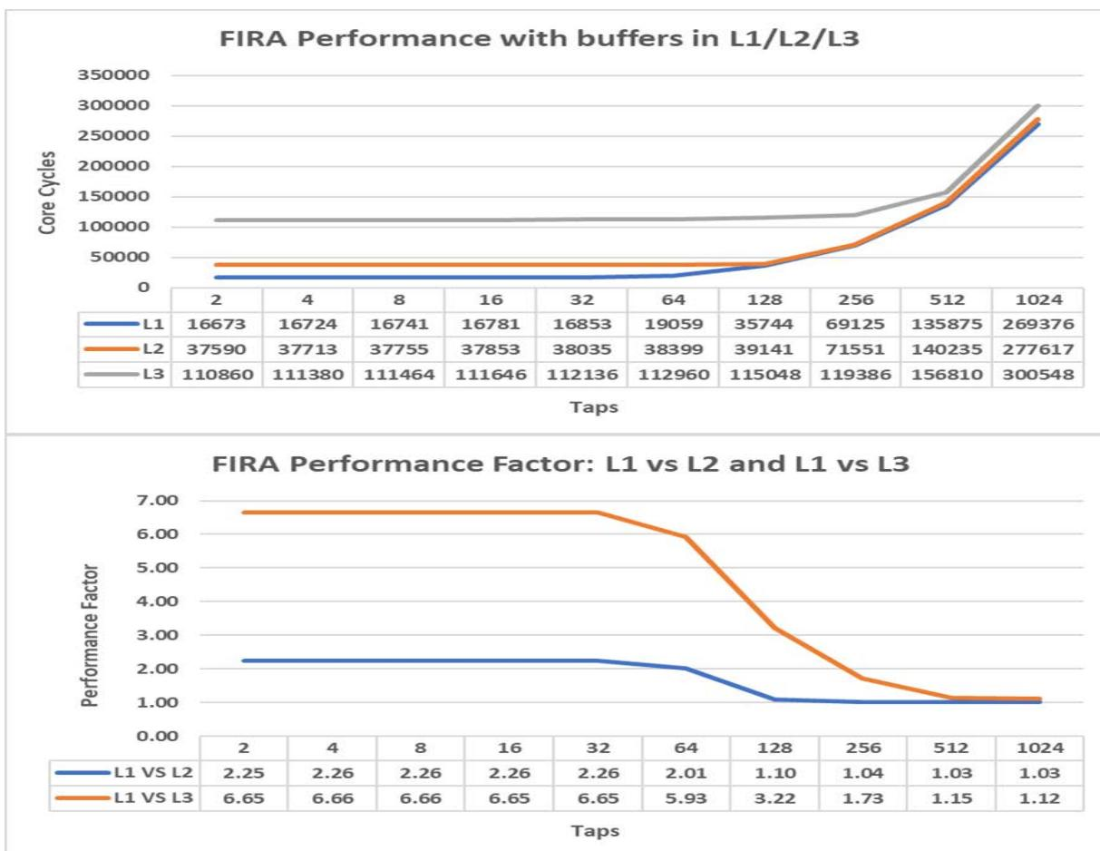
Figure 6: ADSP-2156x FIRA Performance Comparison for Buffers in L1/L2/L3 Memory
