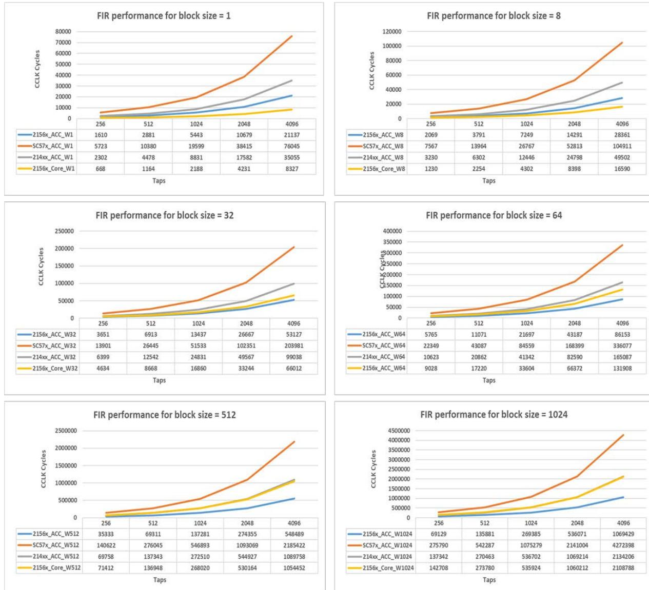
*Figure 2: FIR Performance in Core Cycles Across Window Size and Tap Length*
