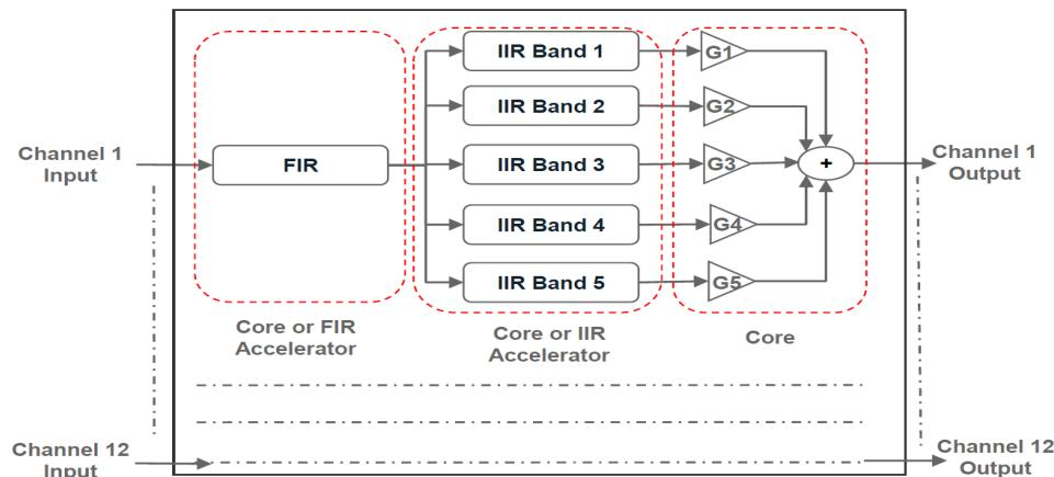
Figure 14: FIR/IIR Real-Time Use Case
