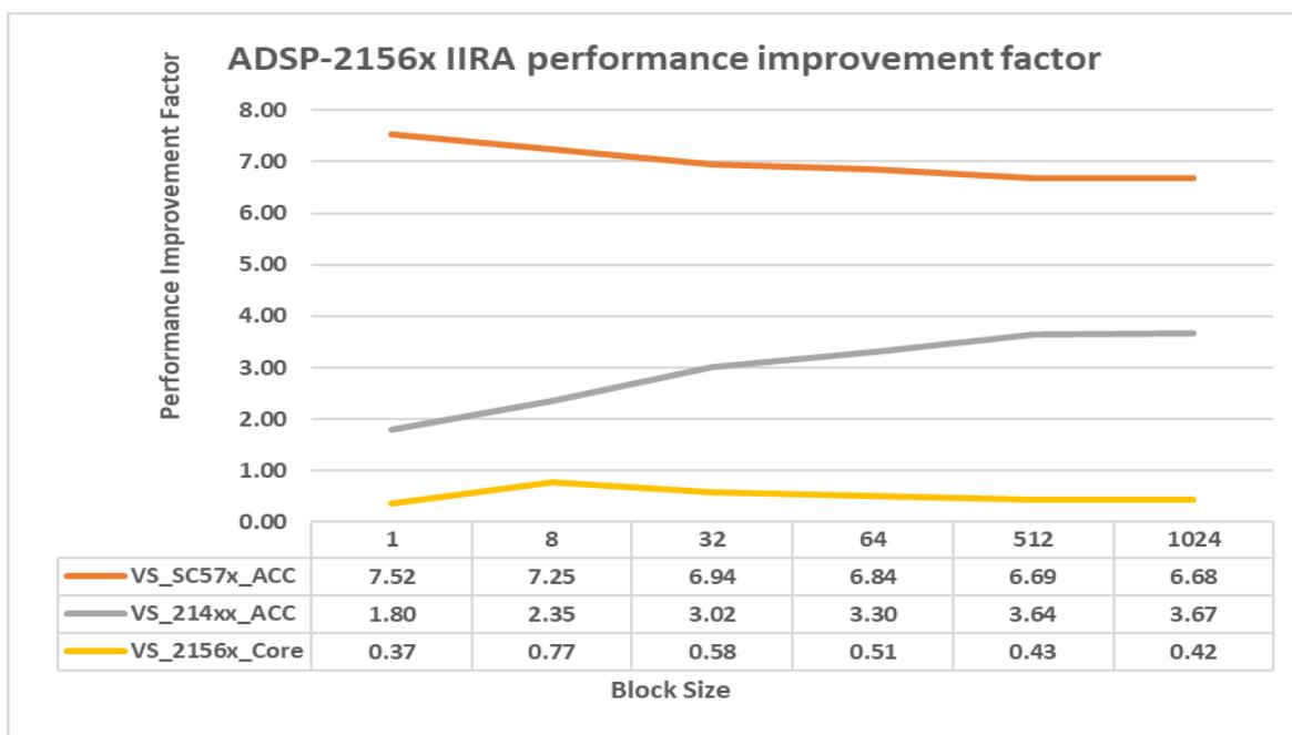
Figure 9: ADSP-2156x IIR Performance Improvement Factor for 6 Biquads Considering Time
