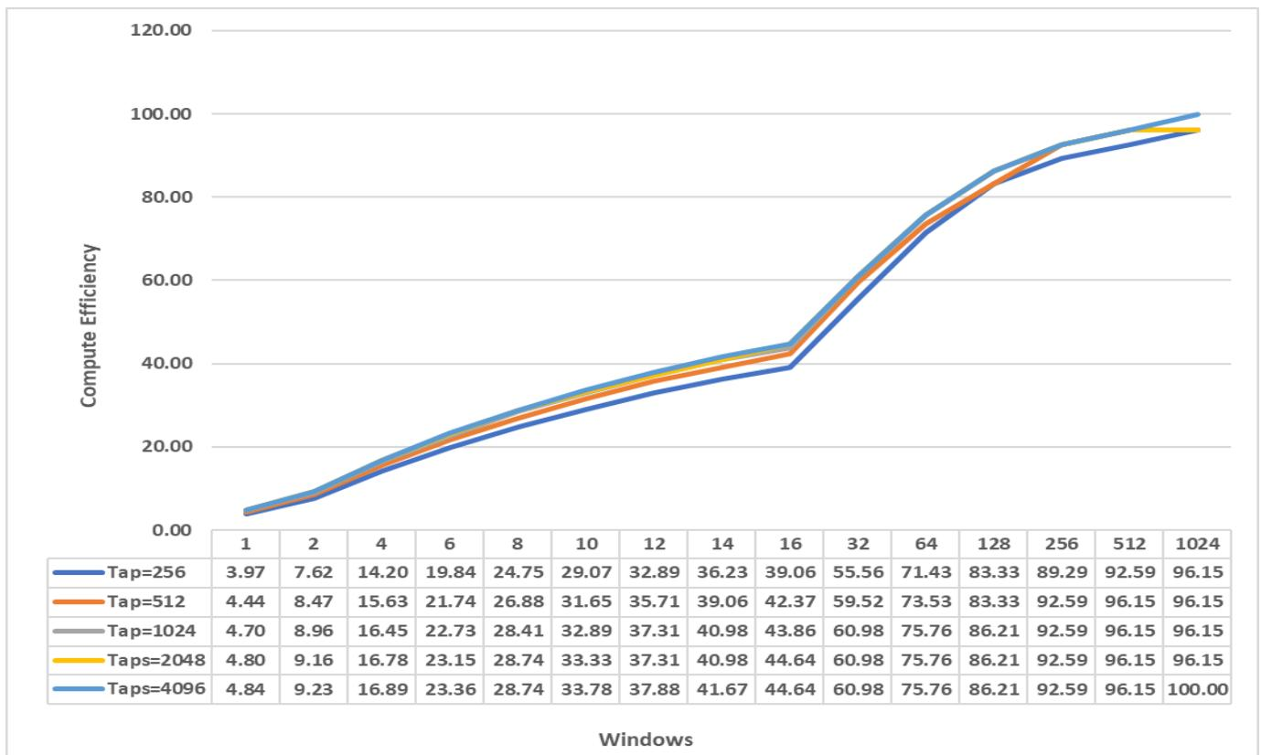
Figure 5: FIRA Compute Efficiency (CE) for Different Filter Parameters
