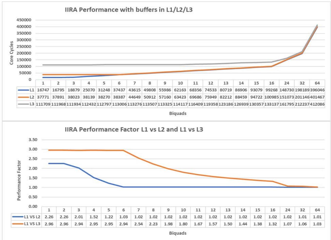
Figure 11: ADSP-2156x FIRA Performance Comparison for Buffers in L1/L2/L3 Memory
