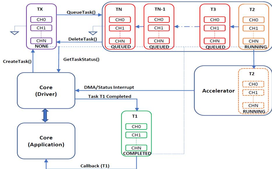
Figure 12: ADSP-2156x Accelerator Device Driver Structure
