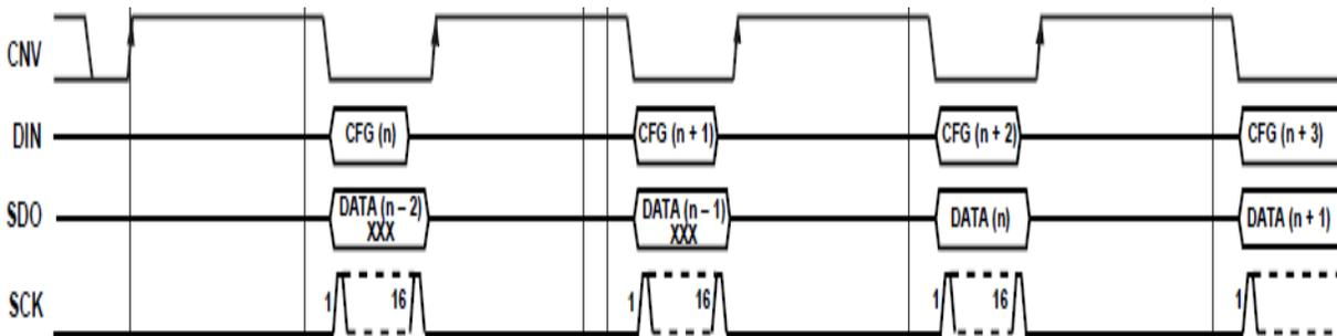
Figure 3 Read/Write After Conversion Timing Diagram
