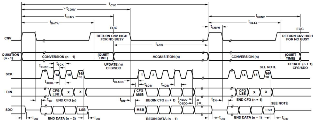
Figure 2 Read/Write During Conversion Timing Diagram
