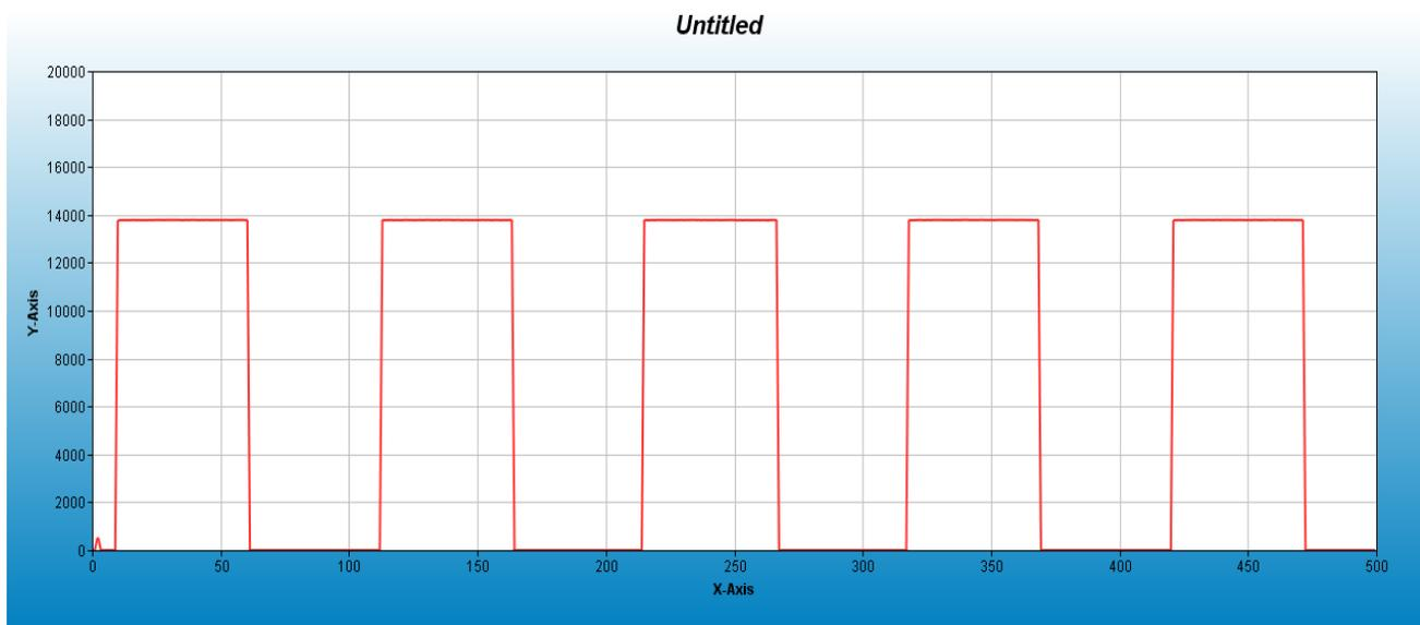
Figure 5 Square Wave (2 kHz, 500 mV) Output from ADC
