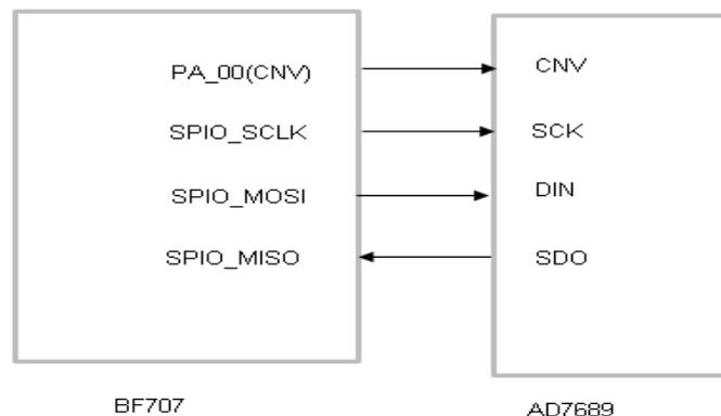
Figure 1. ADSP-BF70x/AD7689 SPI Interface
