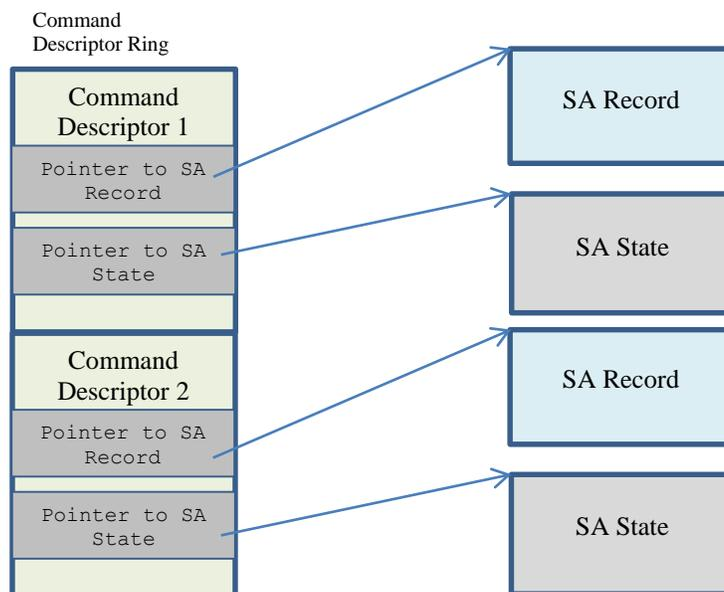
Figure 3. Representation of Command Descriptor Ring
