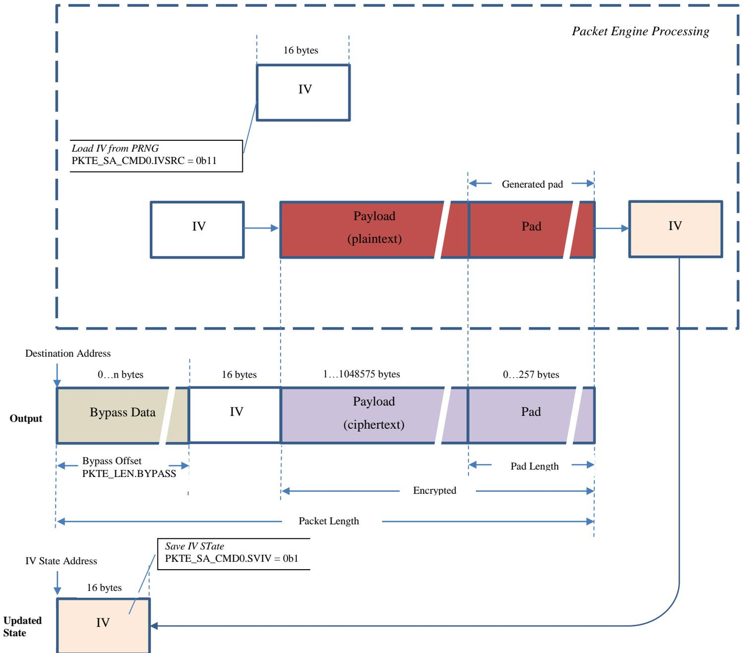
Figure 2. Data Consumption and Output Data Formatting by Security Packet Engine
