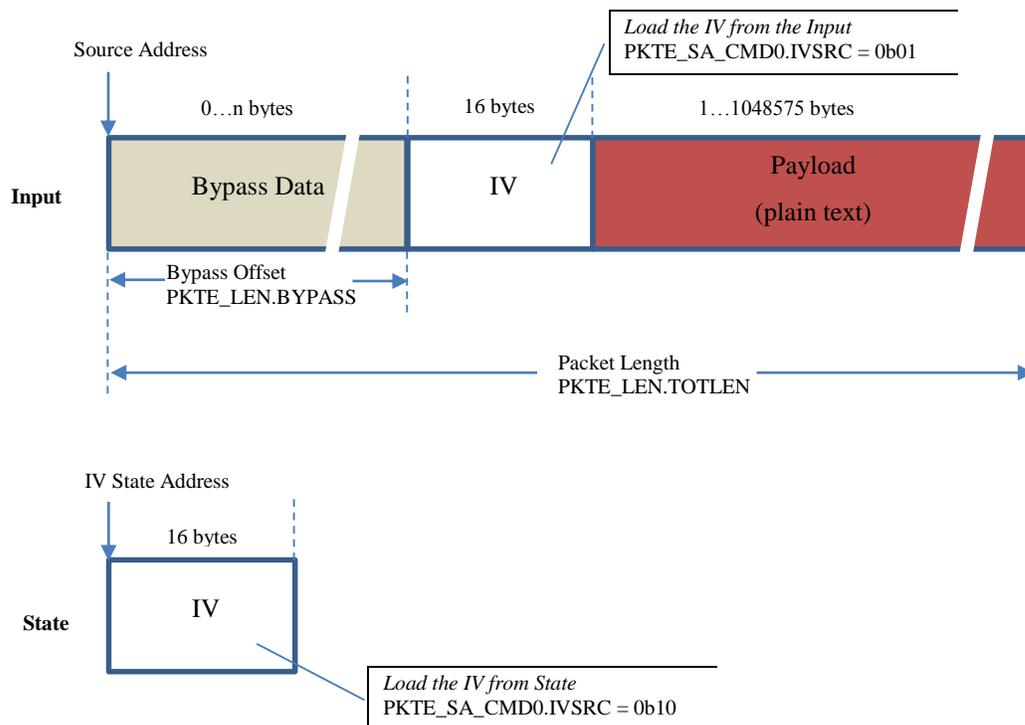
Figure 1. Input Data Formatting for the Security Packet Engine
