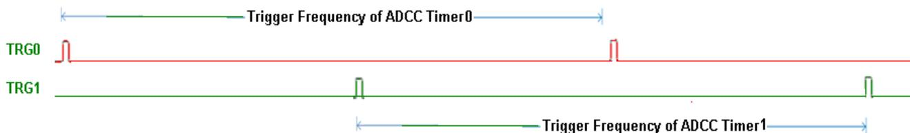
Figure 6. ADCC timer triggers
