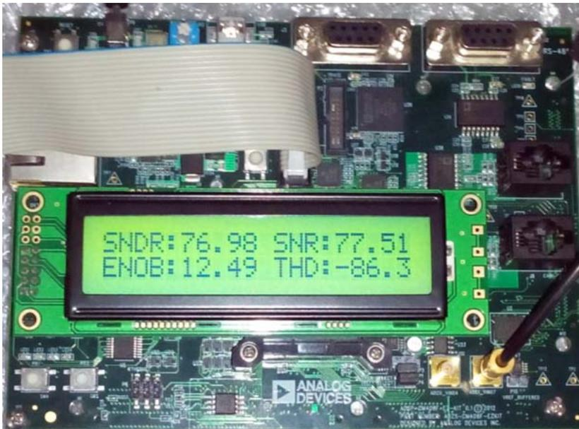
Figure 8. ADC performance measurements results
