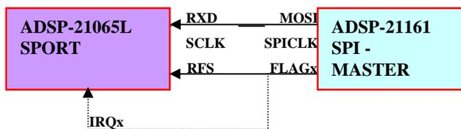
Figure 2. Gated Clock Setup of the SPORT
