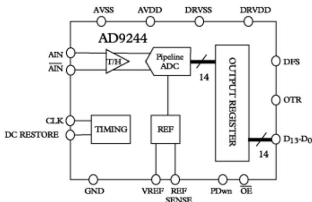
Figure 1. AD9244 Block Diagram
