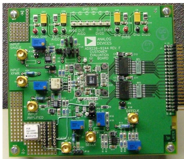
Figure 2. AD9244 ADC Evaluation Board
