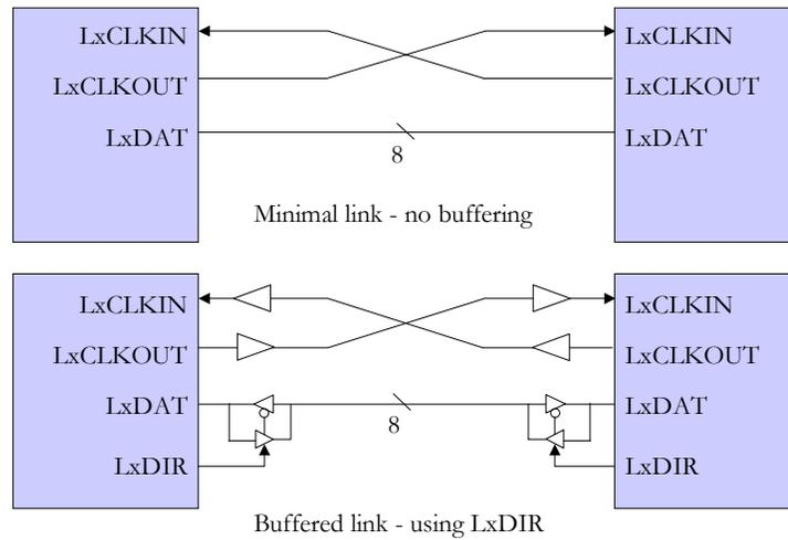
Figure 6. Buffered link port configuration
