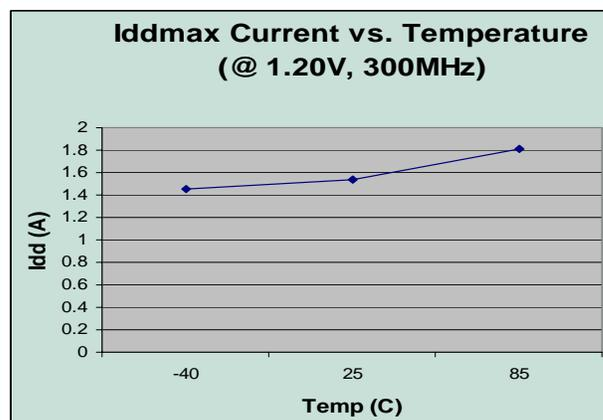
Figure 2:  $I_{DDMAX}$  Current vs. Temperature
