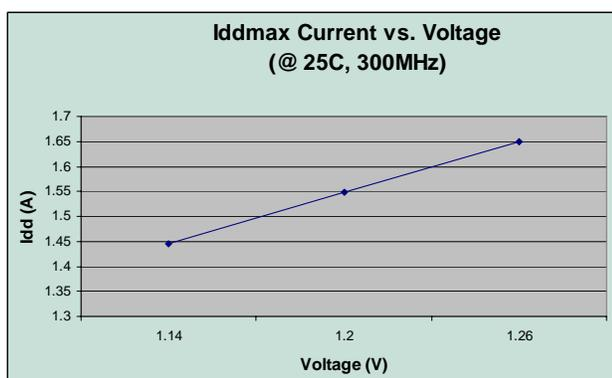
Figure 1:  $I_{DDMAX}$  Current vs. Voltage
