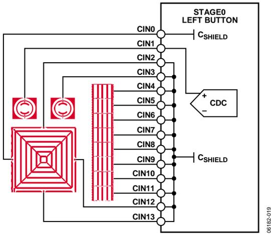
Figure 19. Stage0 Connections, Left Button Connected to CDC
