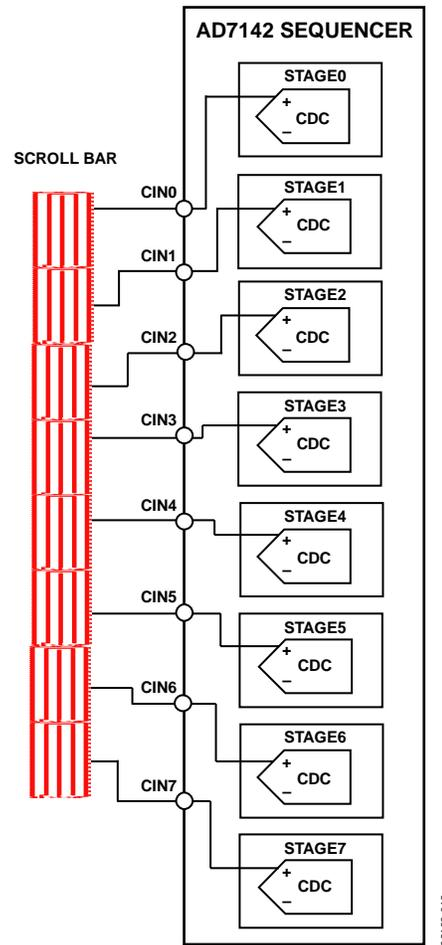
Figure 12. Discrete Slider Connection to the AD7142/AD7143 and CDC (AD7142 Shown)
