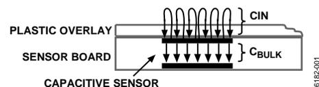
Figure 1. Sensor Bulk Capacitance and Fringe Capacitance
