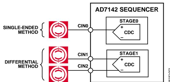
Figure 3. Methods for Connecting Buttons to the AD7142/AD7143 and the CDC (AD7142 Shown)
