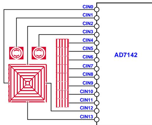
Figure 18. Sensor Connections to the AD7142/AD7143 (AD7142 Shown)
