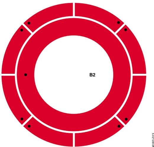
Figure 13. Scroll Wheel Sensor Layout
