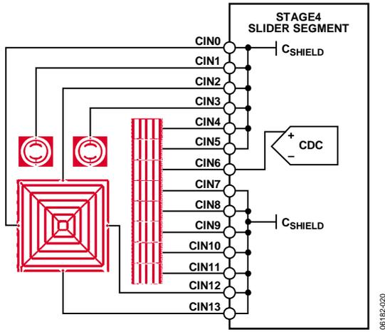
Figure 20. Stage4 Connections, Slider Segment 3 Connected to CDC
