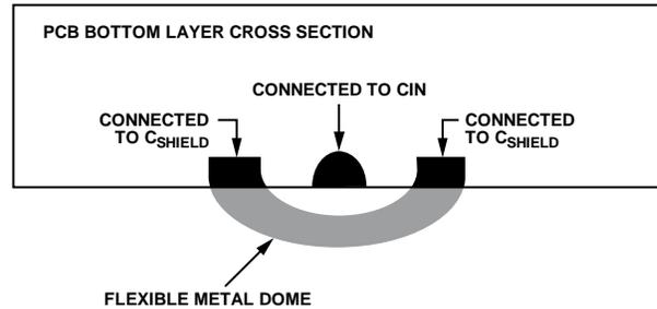
Figure 8. Mechanical Button Construction
