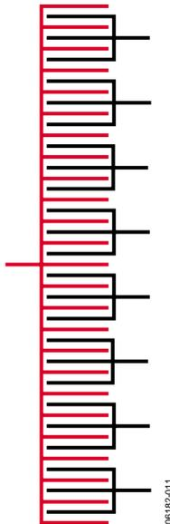
Figure 11. Discrete Slider Sensor Layout
