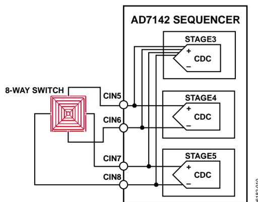
Figure 10. 8-Way Switch Connection to AD7142/AD7143 and CDC
