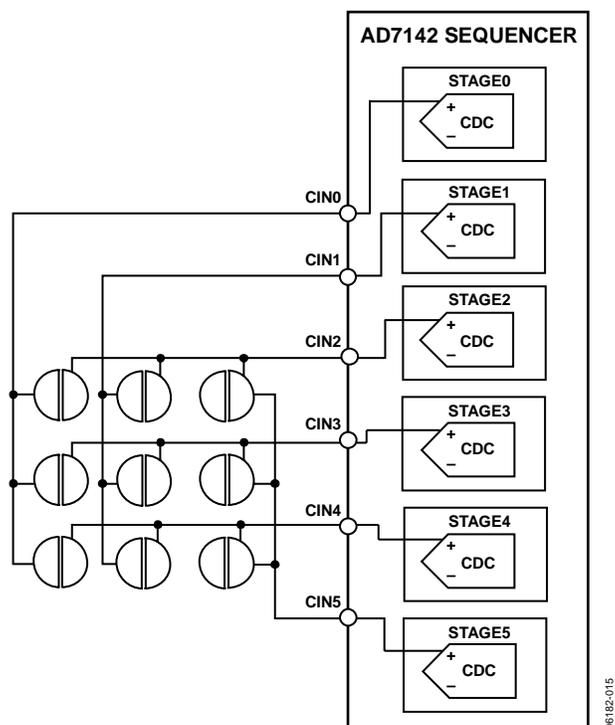
Figure 15. 3 × 3 Matrix Keypad Connection to the AD7142/AD7143 and CDC (AD7142 Shown)
