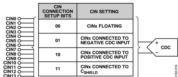
Figure 16. CIN Connection Setup Bits
