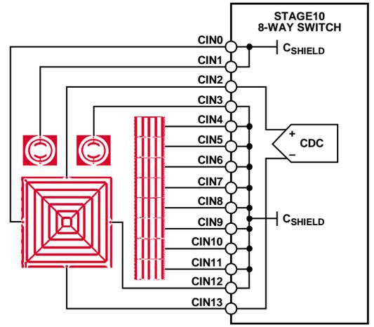
Figure 21. Stage10 Connections, Top and Bottom 8-Way Switch Segments Connected to CDC
