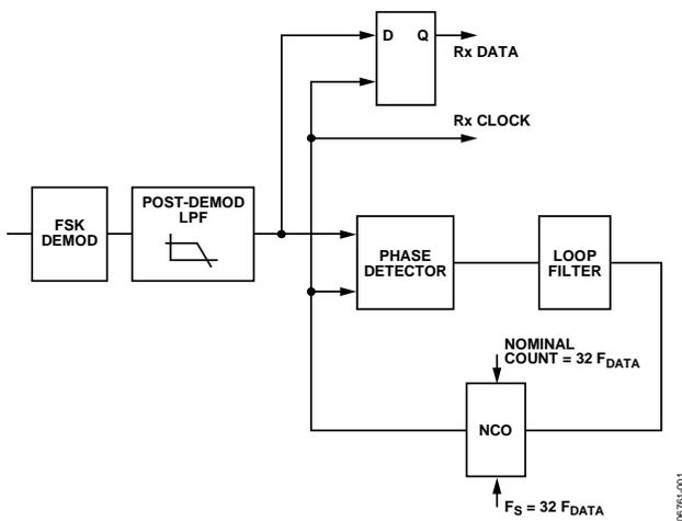
Figure 1. Block Diagram of Symbol Timing Recovery PLL
