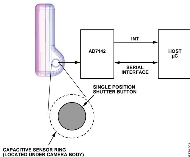
Figure 1. Capacitive Sensor Shutter Button Block Diagram
