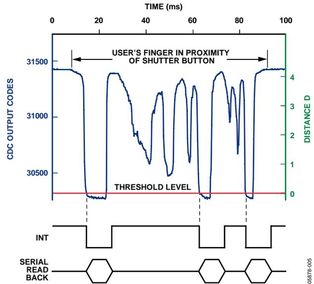
Figure 5. Example of Interrupt Output Timing for Multiple Shutter Button Contacts
