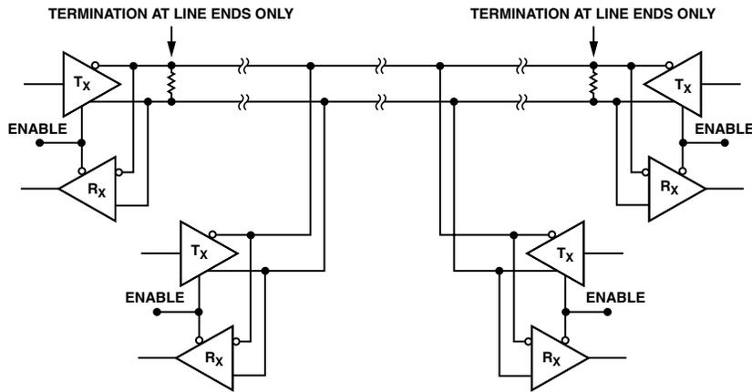
Figure 1. RS-485 2-Wire Multidrop, Half-Duplex Network
