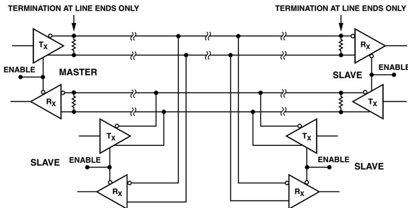
Figure 2. RS-485 4-Wire Multidrop, Full-Duplex Network
