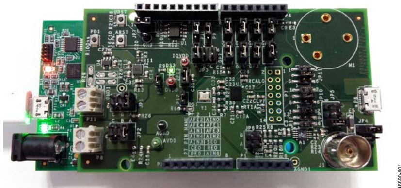
Figure 1. EVAL-AD5940ELCZ Plugged into the EVAL-ADICUP3029
