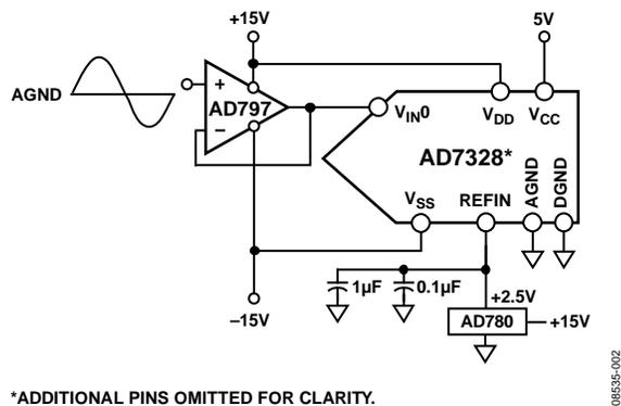
Figure 2. Single-Ended Input Operation (Simplified Schematic: Decoupling and All Connections Not Shown)
