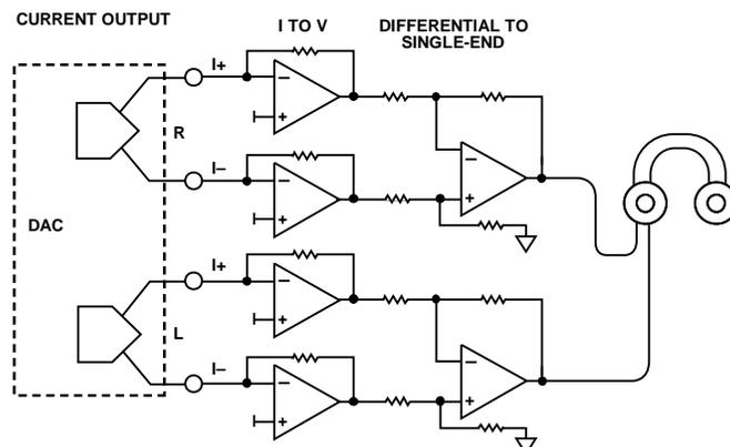
Figure 2. Current Output Configuration
