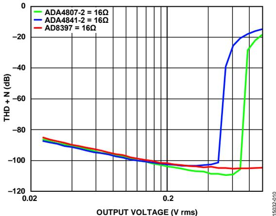
Figure 10. THD+N vs.  $V_{OUT}$  of the [ADA4841-2](#), [ADA4807-2](#), and [AD8397](#)
