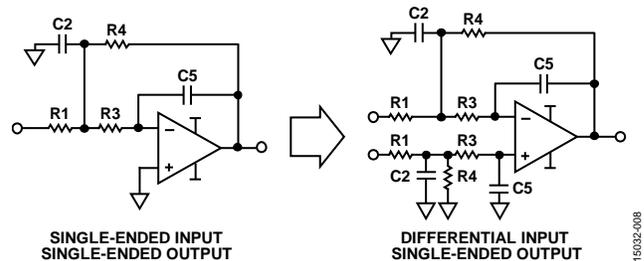
Figure 8. Second-Order Multiple Feedback (MFB) Filter
