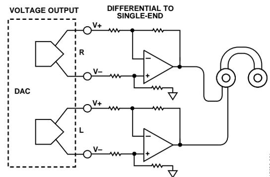
Figure 1. Voltage Output Configuration
