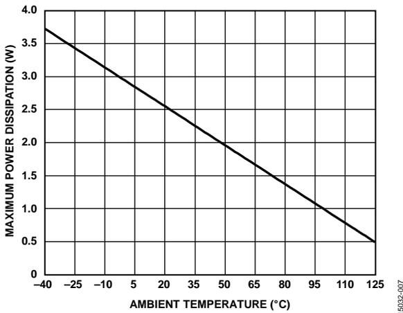
Figure 7. ADA4807-2 Maximum Power Dissipation vs. Ambient Temperature for a 4-Layer Evaluation Board
