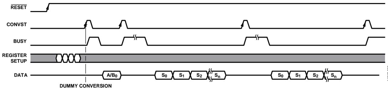
Figure 5. Burst Mode Operation
