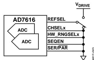
Figure 3. Hardware Control Pin Connections
