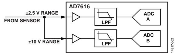
Figure 2. Dual Gain Sampling Setup
