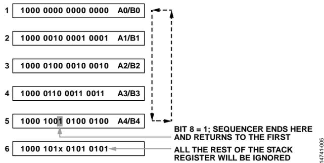
Figure 5. Programming the AD7616 Sequencer to Activate a Sampling Burst
