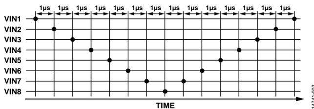
Figure 2. Analog Channel VINx Sampling Pattern
