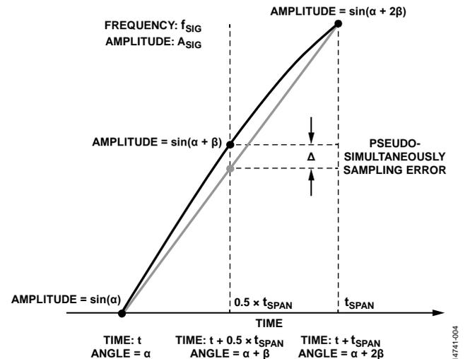
Figure 4. Determining Sampling Error
