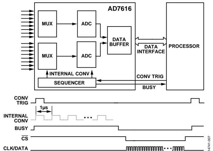
Figure 7. Sampling Burst Achieved by Using the Burst Mode of the AD7616
