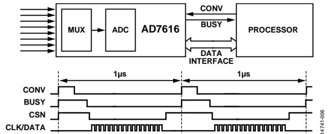
Figure 6. Sampling Burst Achieved by Using a Traditional Muxed Input ADC
