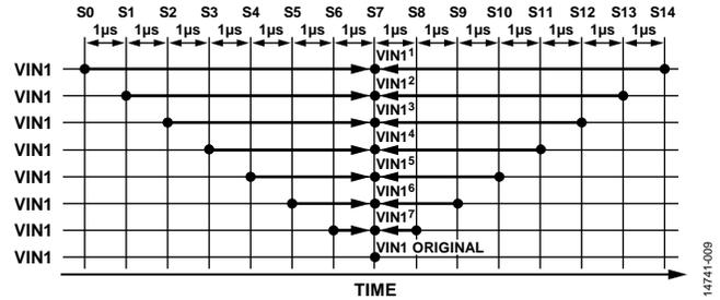
Figure 9. VIN1 Sample (S0 to S14)
