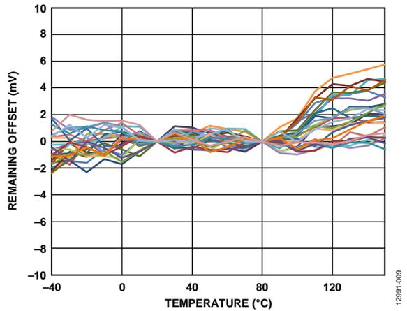
Figure 10. Sine and Cosine Remaining Offset After a Two-Point Calibration at 20°C and 80°C
