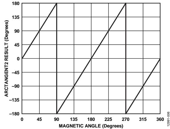
Figure 7. Calculated Angle over an Entire Mechanical Revolution
