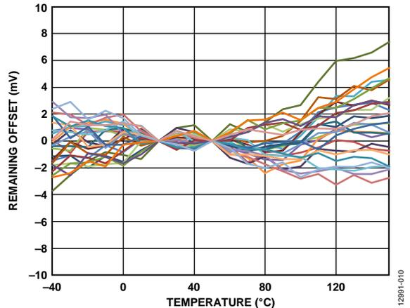
Figure 11. Sine and Cosine Remaining Offset After a Two-Point Calibration at 20°C and 50°C
