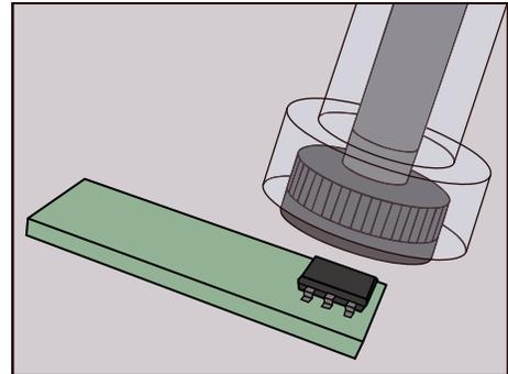
Figure 1. Typical Measurement Configuration for an AMR Angle Sensor
