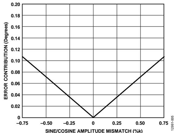
Figure 6. Theoretical Error Contribution due to Amplitude Mismatch of Sine/Cosine Outputs
