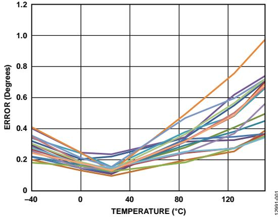
Figure 2. Angular Error over Temperature After Calibration at Room Temperature, GC Enabled
