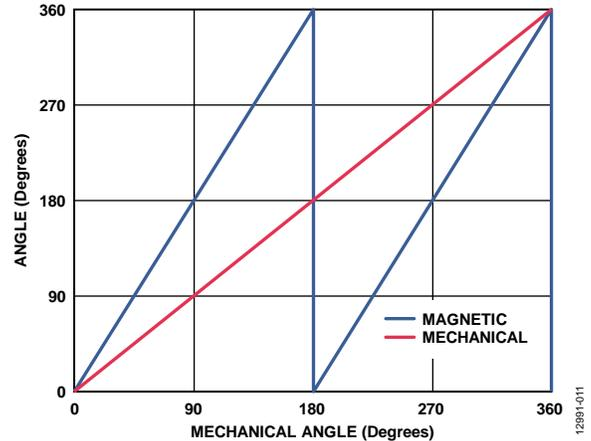
Figure 12. Magnetic vs. Mechanical Angle for End of Shaft Magnet Configuration
