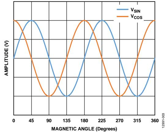
Figure 4. Typical Output Signals over a Single Mechanical Revolution
