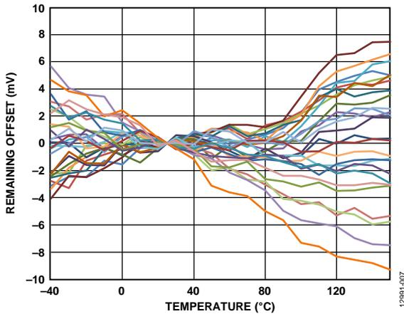
Figure 8. Sine and Cosine Remaining Offset After a Single Point Calibration at 25°C
