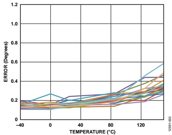
Figure 3. Angular Error over Temperature After Calibration at Room Temperature, GC Disabled
