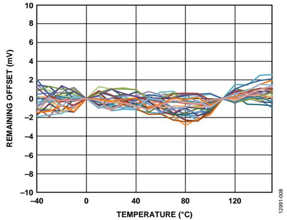
Figure 9. Sine and Cosine Remaining Offset After a Two-Point Calibration at 0°C and 110°C
