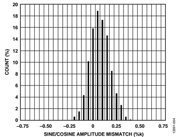
Figure 5. Sample Test Distribution of Sine/Cosine Amplitude Mismatch
