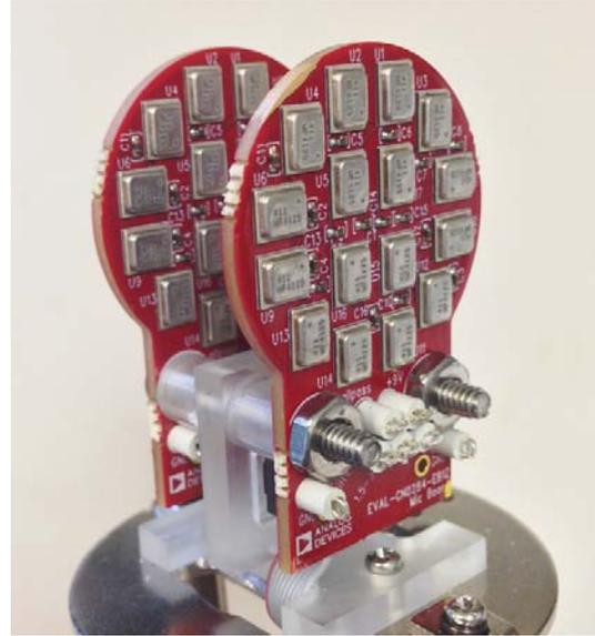
Figure 15. Two Microphone Boards with 18 mm Spacer
