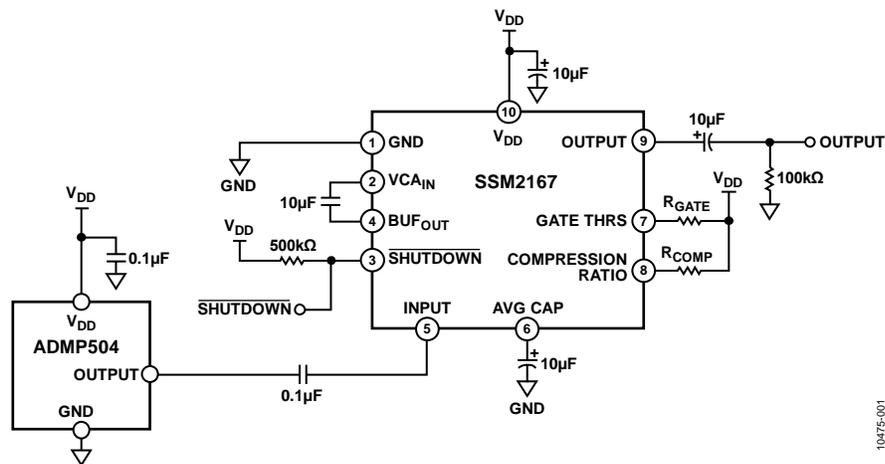
Figure 1. Analog MEMS Microphone Connection to Preamp
