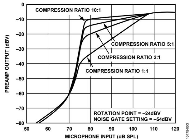
Figure 3. Preamp Output vs. Microphone Input Characteristics
