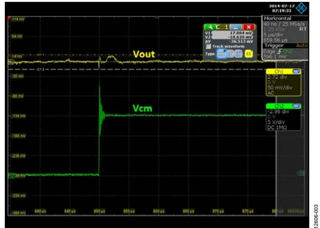
Figure 3. AD8418 Output at Rising Edge
