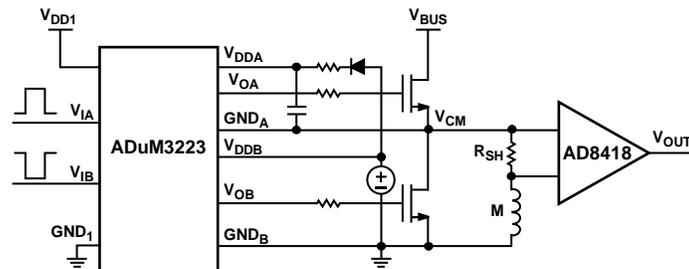
Figure 1. Motor Drive Circuit with the [ADuM3223](#) and the [AD8418](#)
