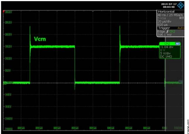
Figure 2. Common-Mode Voltage at the Half-Bridge Point
