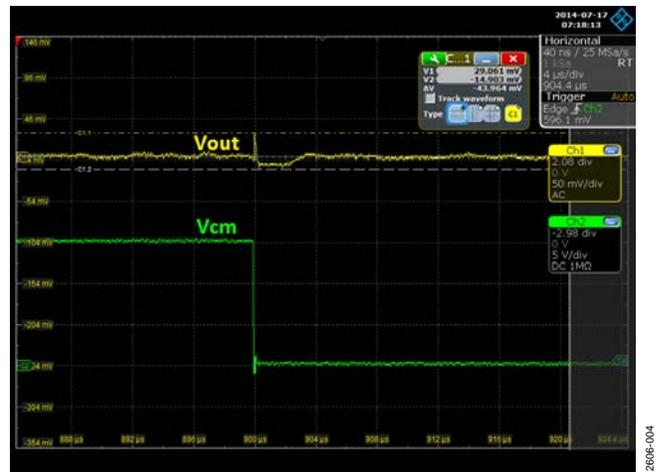
Figure 4. AD8418 Output at Falling Edge
