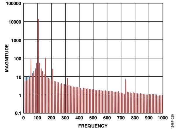
Figure 19. FFT of Misaligned Sensor
