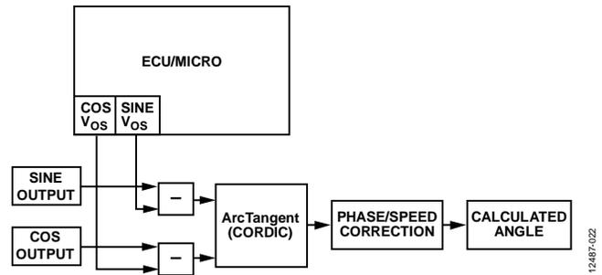
Figure 21. Dynamic Calibration Operating Flow Chart
