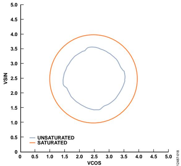
Figure 17. Radius of Unsaturated and Saturated Sensors
