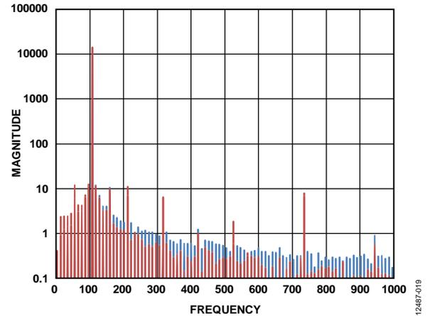
Figure 18. FFT of Well Aligned Sensor
