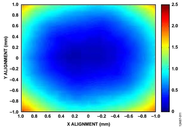
Figure 11. NdFeB (35 MGOe) with 1 mm Air Gap
