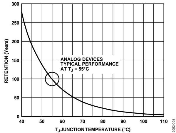
Figure 7. Example of Data Retention vs. Temperature
