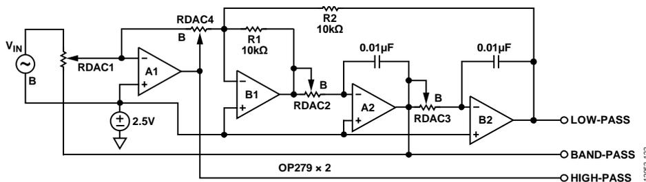
Figure 24. Programmable State Variable Filter
