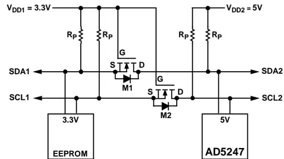
Figure 17. Level Shifting for Operation at Different Potentials
