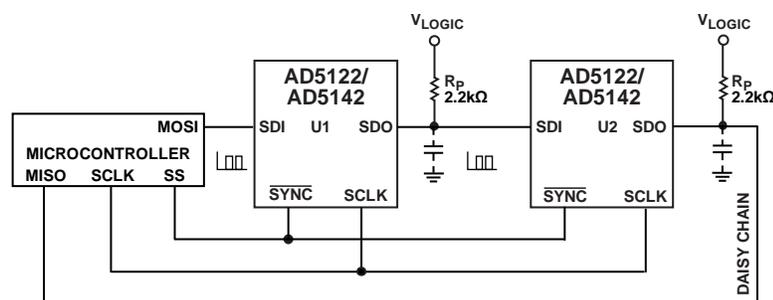
Figure 6. Daisy-Chaining Digital Potentiometers
