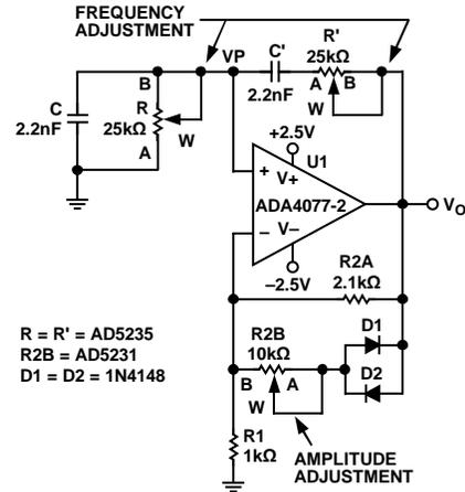
Figure 27. Programmable Oscillator with Amplitude Control
