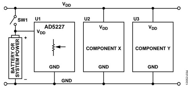
Figure 28. Constant Bias of the AD5227 for Resistance Retention
