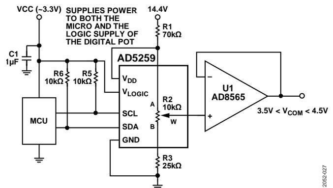
Figure 13. Circuitry When a Separate Supply Is Not Available for the  $V_{DD}$  Pin
