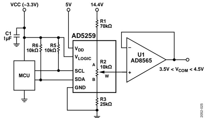
Figure 12.  $V_{COM}$  Adjustment Application
