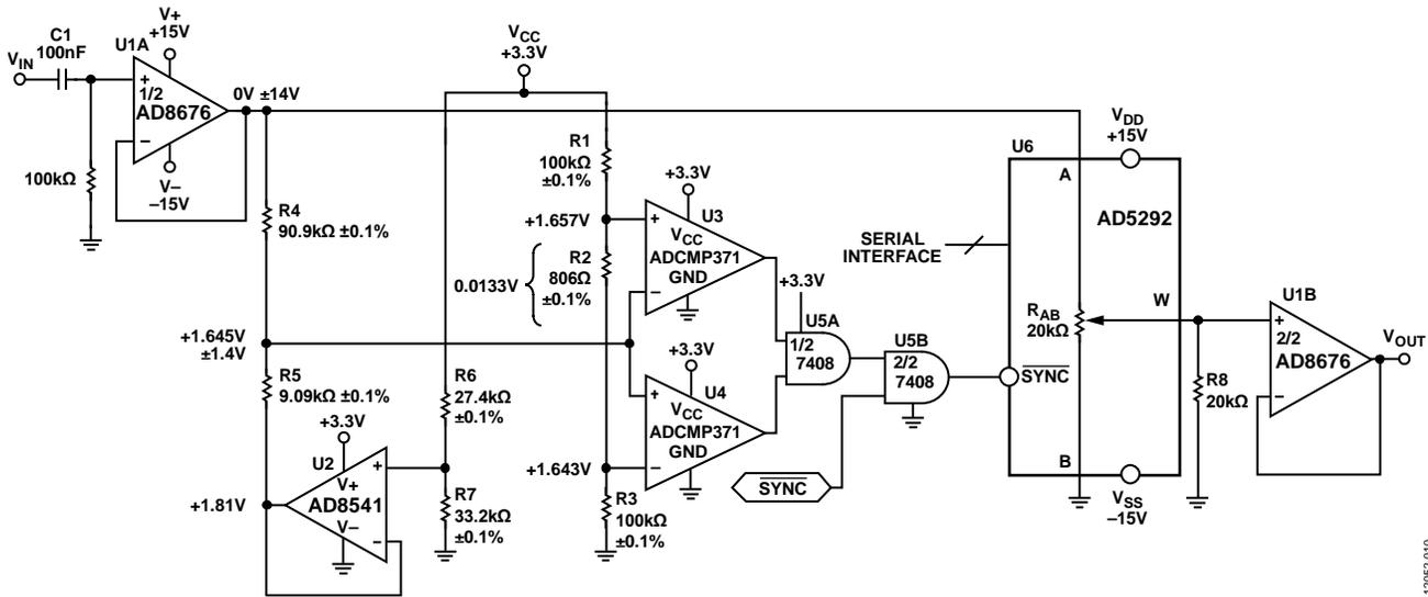
Figure 8. Logarithmic Audio Volume Control with Glitch Reduction (Simplified Schematic; Decoupling; All Connections Not Shown)
