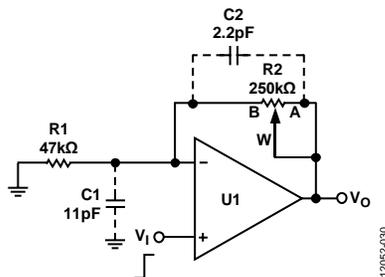
Figure 18. Gain Control Compensation
