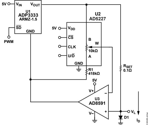
Figure 20. Adjustable Current Source for LED Driver
