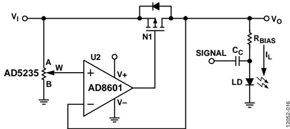
Figure 25. Programmable Booster Voltage Source
