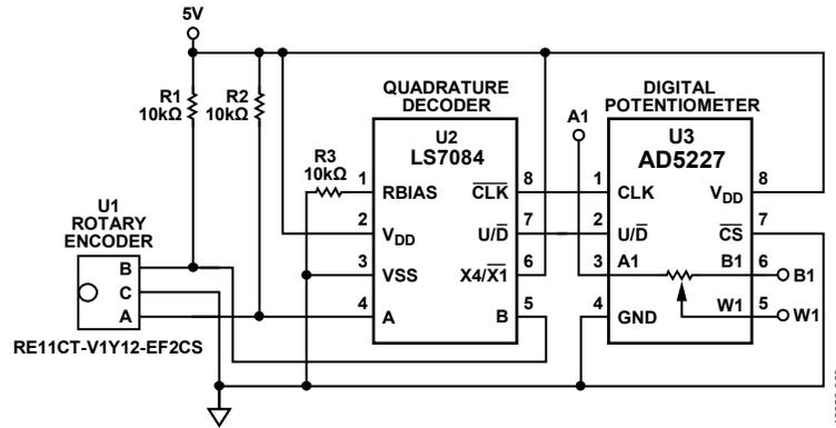
Figure 14. Manual Rotary Control
