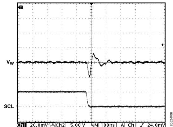
Figure 5. Digital Feedthrough
