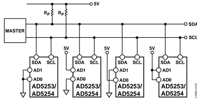
Figure 16. Multiple AD5253/AD5254 Devices on a Single Bus
