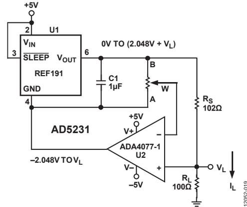
Figure 21. Programmable Current Source
