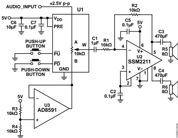
Figure 11. Audio Amplifier with Volume Control
