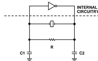
Figure 1. Oscillator Block Diagram
