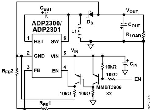
Figure 9. Level Shifting Circuit for the Enable Input
