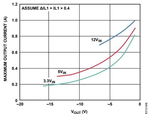
Figure 6. Approximate Application Space for Common Input Voltages
