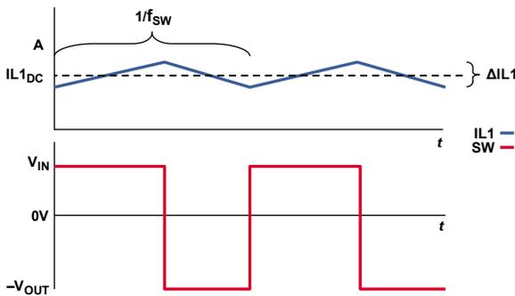
Figure 5. Ideal Current and Voltage Waveforms
