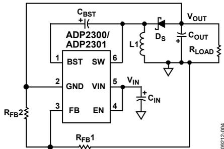
Figure 4. Inverting Buck Boost Topology As Implemented with the ADP230x
