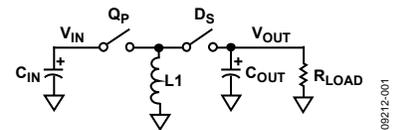
Figure 1. Inverting Buck Boost
