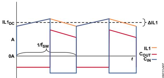
Figure 7. Ideal Current Waveforms for Inductor, C<sub>OUT</sub>, and C<sub>IN</sub>
