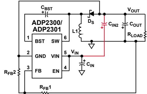
Figure 8. Inverting Buck Boost Topology with V<sub>IN</sub> to V<sub>OUT</sub> Connected Capacitor
