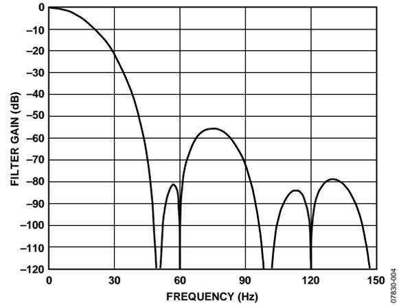
Figure 4. Sinc<sup>4</sup> Filter Response ( $f_{ADC} = 50$  Hz, REJ60 = 1)
