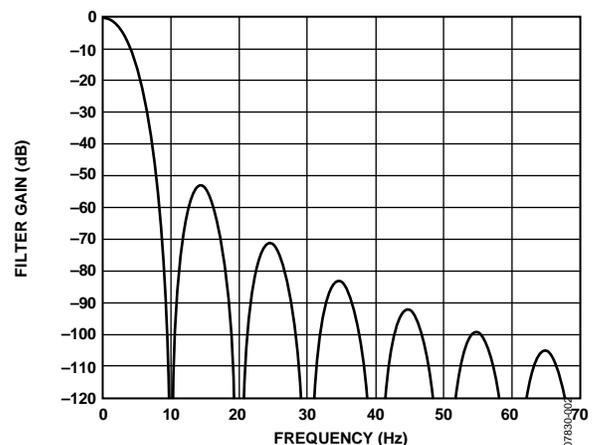
Figure 2.  $\text{Sinc}^4$  Filter Response ( $f_{ADC} = 10$  Hz)
