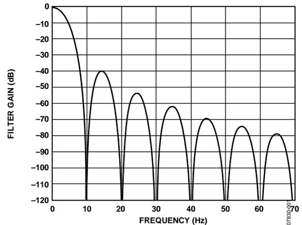
Figure 1.  $\text{Sinc}^3$  Filter Response ( $f_{ADC} = 10$  Hz)
