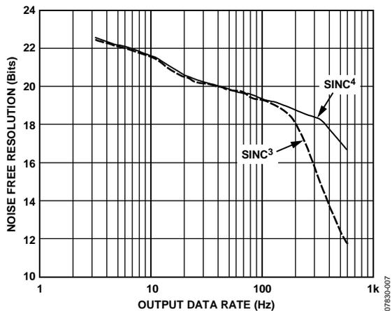
Figure 7. Noise-Free Resolution vs. Output Data Rate (Gain = 1, V<sub>REF</sub> = 5 V)
