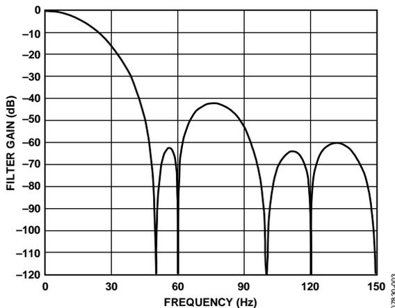
Figure 3. Sinc<sup>3</sup> Filter Response ( $f_{ADC} = 50$  Hz, REJ60 = 1)
