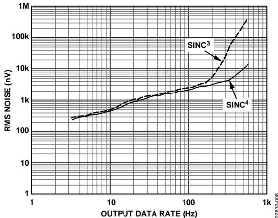
Figure 6. RMS Noise vs. Output Data Rate (Gain = 1, V<sub>RFE</sub> = 5 V)
