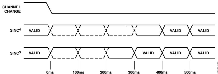
Figure 8. Settling Time (Synchronous Step Change)
