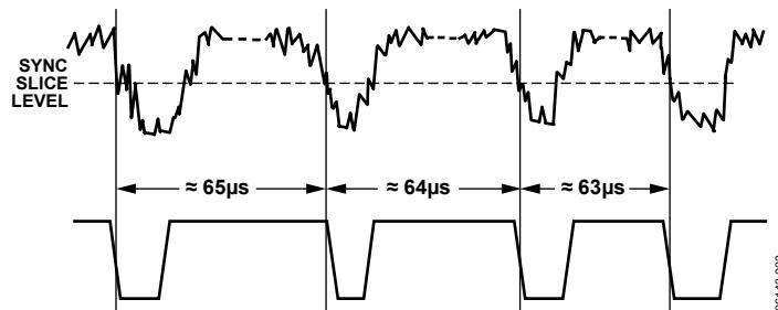
Figure 4. HSYNC Jitter Resulting in Line-to-Line Shifting of Displayed Image
