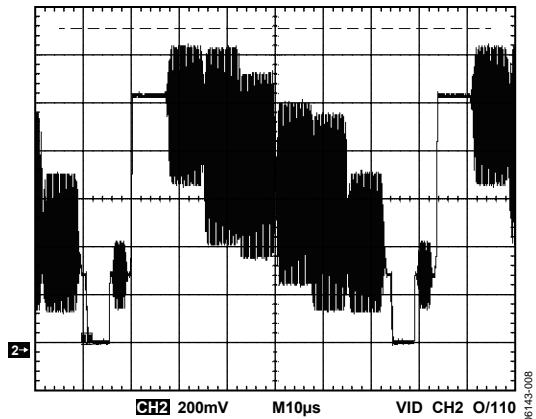
Figure 8. Output Video Signal with Correct Synchronization Level Restored
