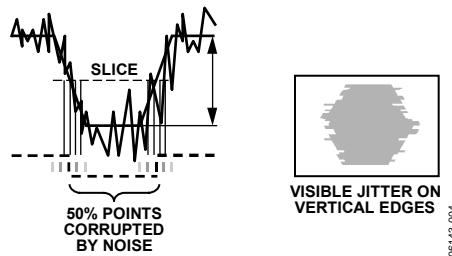
Figure 3. Noisy Synchronization Information Resulting in Extracted Synchronization Jitter
