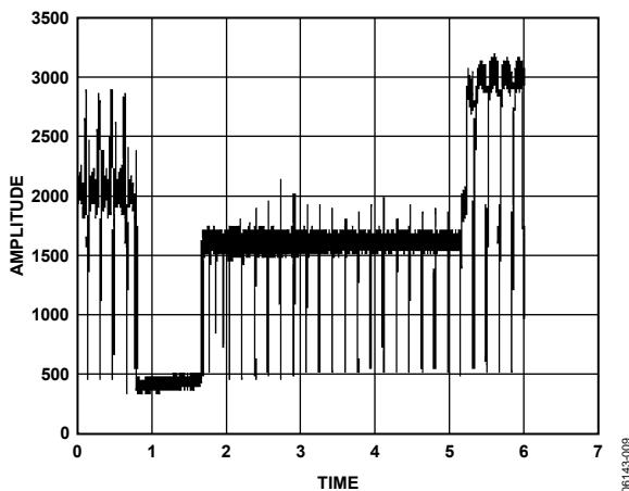
Figure 9. VCR Missing Signal During Head Switch
