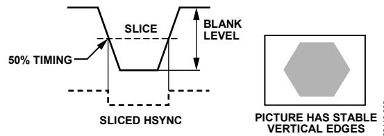
Figure 2. Stable Synchronization Extraction with No Vertical Jitter on Displayed Image
