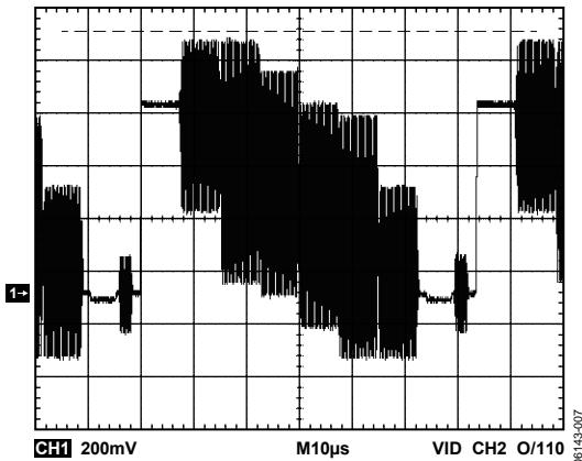
Figure 7. Input Video Signal with Attenuated Synchronization
