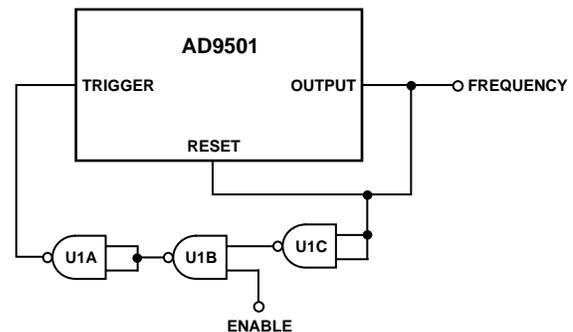
Figure 8. The AD9501 Configured as a Programmable Oscillator
