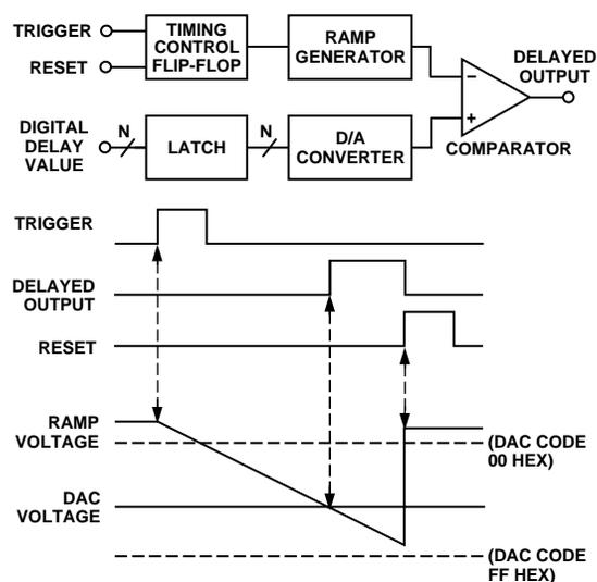
Figure 2. Delay Generator Block Diagram and Basic Timing
