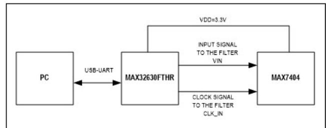
Figure 2. Block diagram
