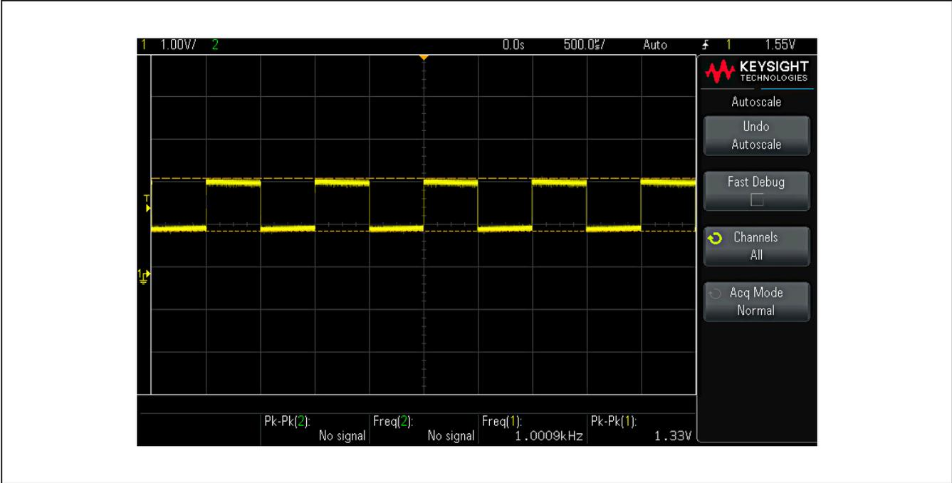
Figure 4. Input square wave to the filter.
