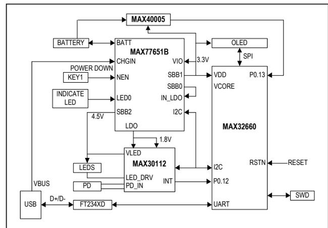
Figure 2. MAXREFDES1207 block diagram.
