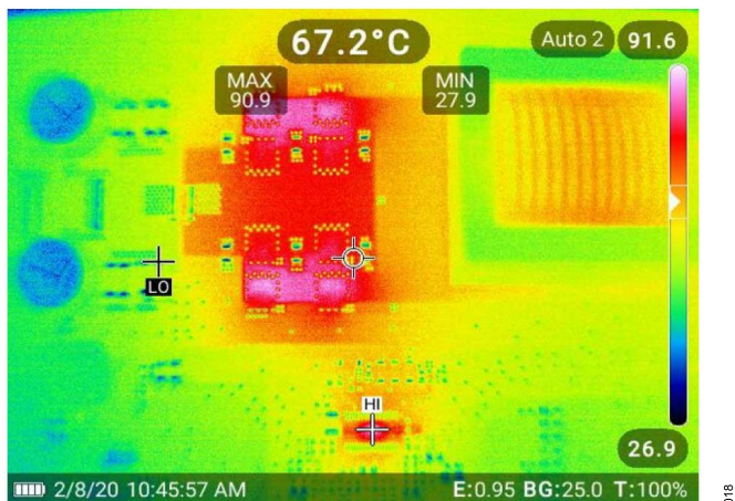
Figure 18. CN0556 Boost Mode Thermal Performance
