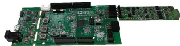
Figure 7. EVAL-CN0531-PMDZ Connected to EVAL-ADICUP3029
