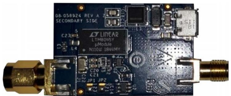
Figure 13. Bottom View of the EVAL-CN0522-EBZ
